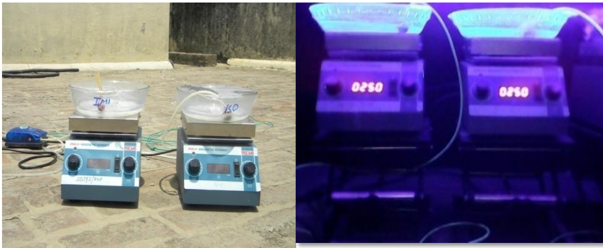
Figure 4.5: Reaction vessel in (a) In Solar light (b) In UV light
