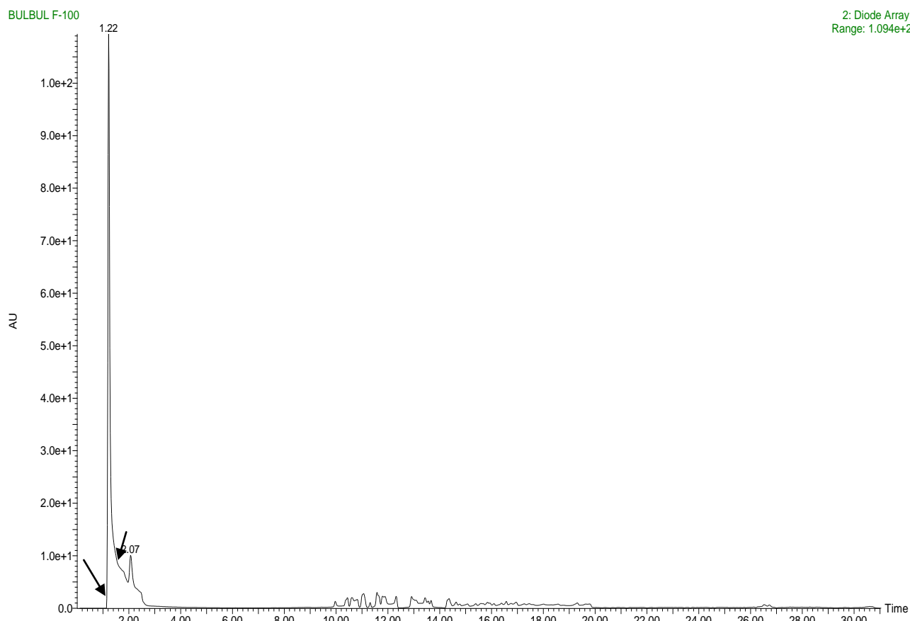
Figure 4.16: Chromatogram of Naphthalene standard (100µg/g) after 7 day of incubation with F3.
