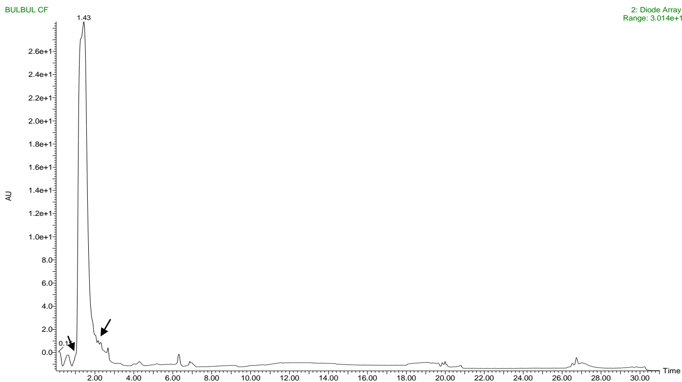
Figure 4.18: Chromatogram of Contaminated Soil after 7 days of incubation with F3 strain.
