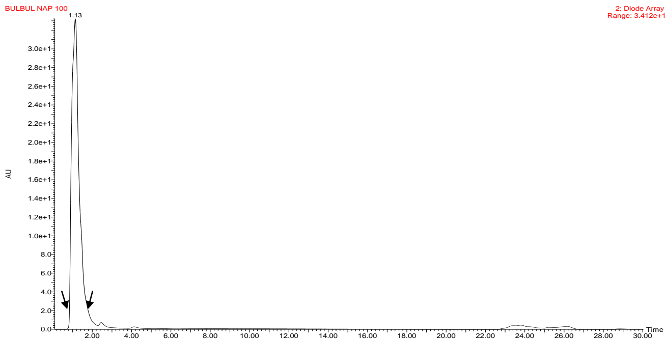
Figure 4.8: Chromatogram of Naphthalene standard (100µg/g) at 0 day of incubation.
