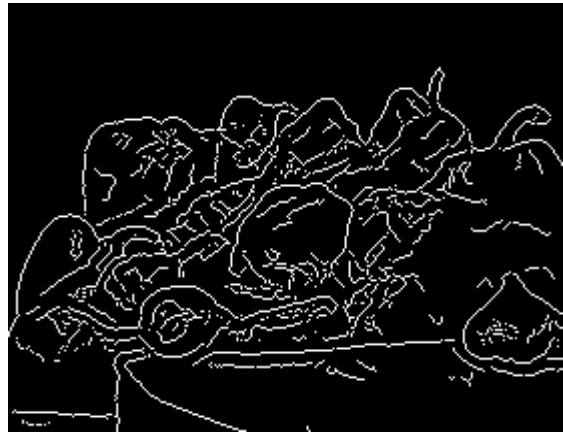
Figure-5.52: Canny Edge Detected Image, t_2=0.10 , t_1=0.04 , \sigma=1.5
