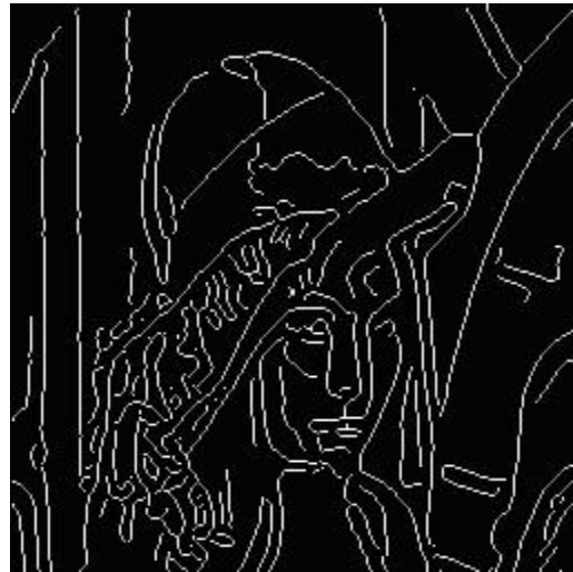
Figure-5.42: Canny Edge Detected Image, t_2=0.10 , t_1=0.04 , \sigma=1.5
