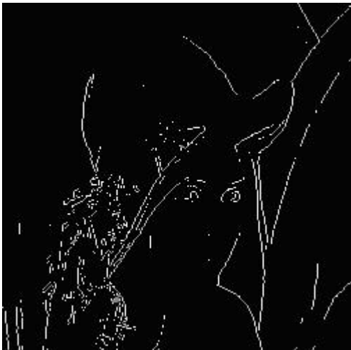
Figure-5.45: Sobel Edge Detected Image, t=0.15
