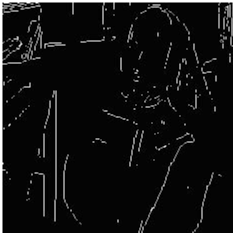
Figure-5.35: Sobel Edge Detected Image, t=0.15
