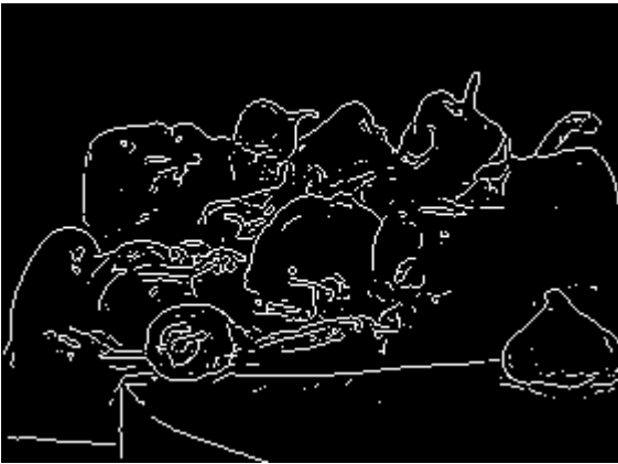
Figure-5.55: Sobel Edge Detected Image, t=0.05
