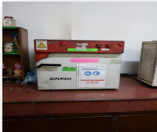
Figure 3.10 Standard equipment for ageing test (Source: Vibracoustic India Pvt. Ltd. Mohali)
