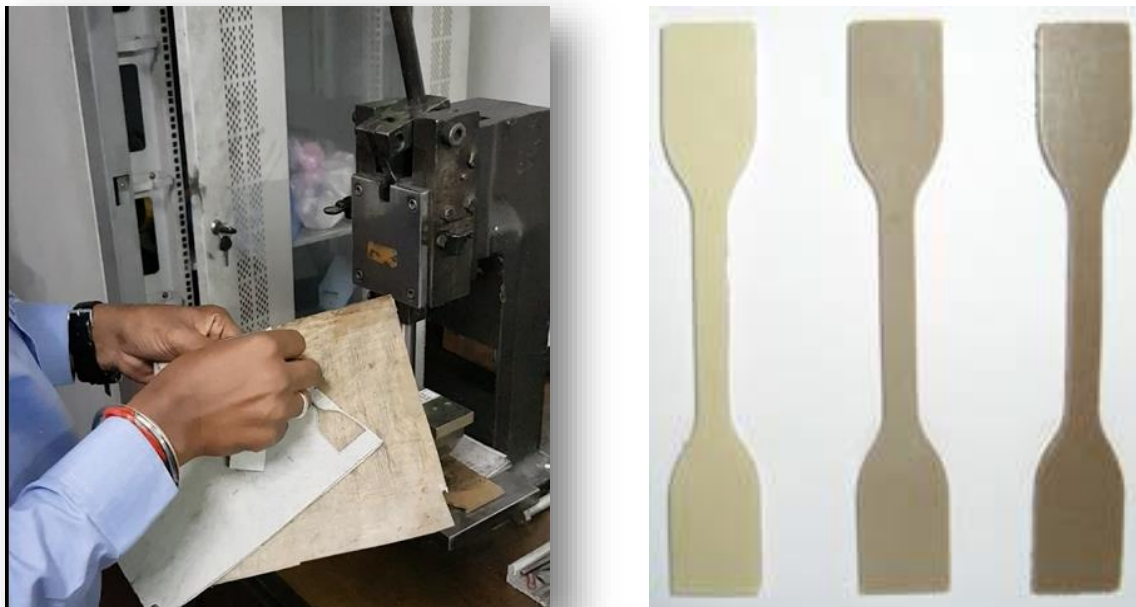
Figure 3.7 Dumbbell or dog bone shape of EPDM nanocomposite cuttings
