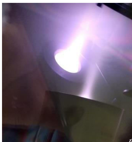
Fig. 2.5: Photograph of the plasma during the co-sputtering from RF and DC targets
