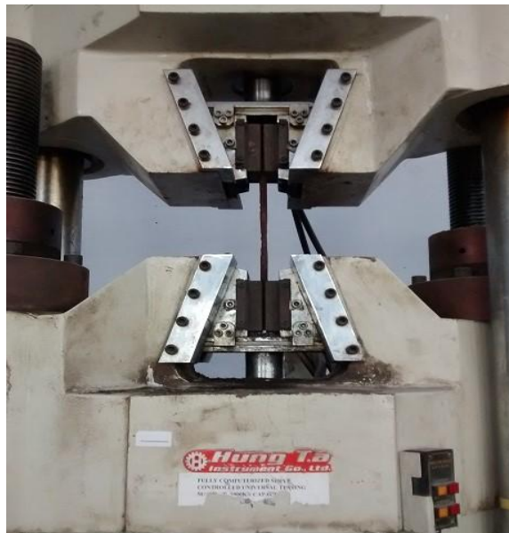
Figure 4.9: Tensile testing of corroded steel bar specimen.
