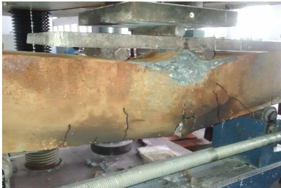
Figure 4.6: Observed failure mode of beam B5.
