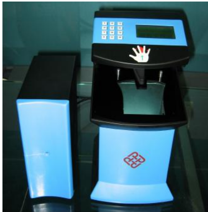
Figure 2.3: A CCD-based palmprint scanner
