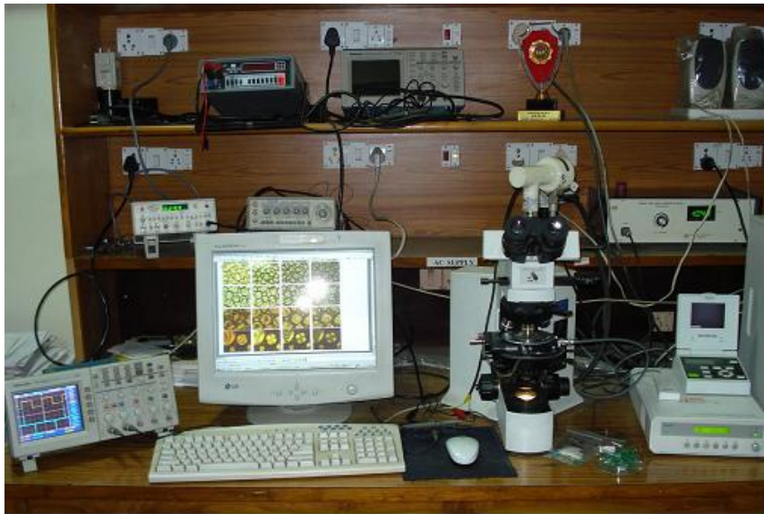
Figure 2.4: Optical polarizing microscope and thermo-optical set up
