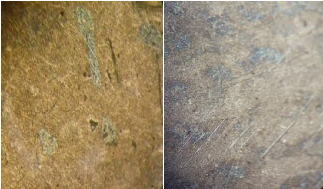
Figure 7.5 Microstructure of LM6, Pouring Temperature 770 0 , and Injection pressure 180 Kg/cm 2 , Dycot Coating, Air Cooling.
