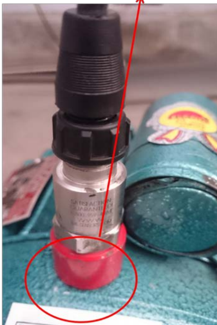
Figure 3.2- Vibration signal acquisition using CESVA SC310
