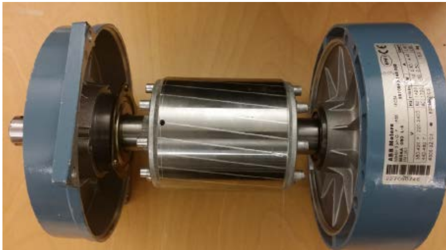
Figure 2.5- Broken rotor bar fault introduced in squirrel cage [2]
