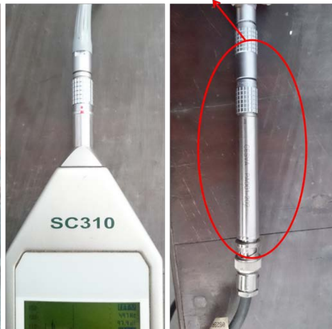
Figure 3.2- Vibration signal acquisition using CESVA SC310
