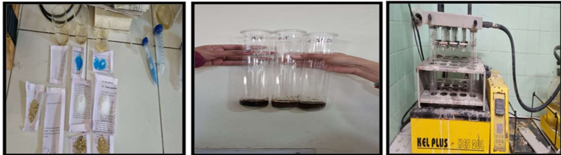
Fig9. Kjeldahl nitrogen estimation apparatus for protein content determination of the seed sample.
