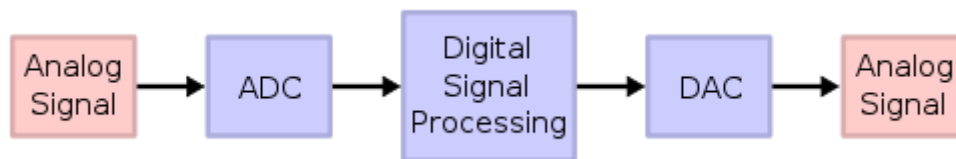
Figure 1.2 - Digital signal processing scheme
