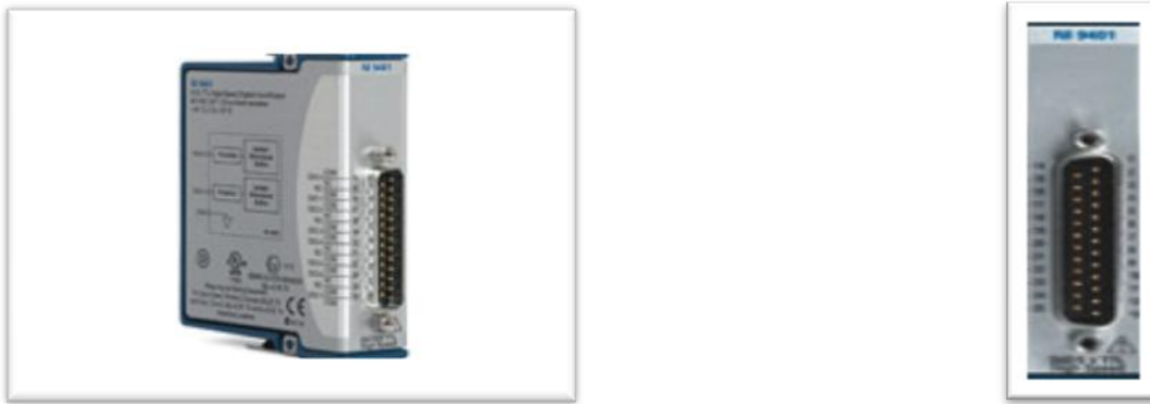
Figure 4.10: NI 9401 digital I/O module
