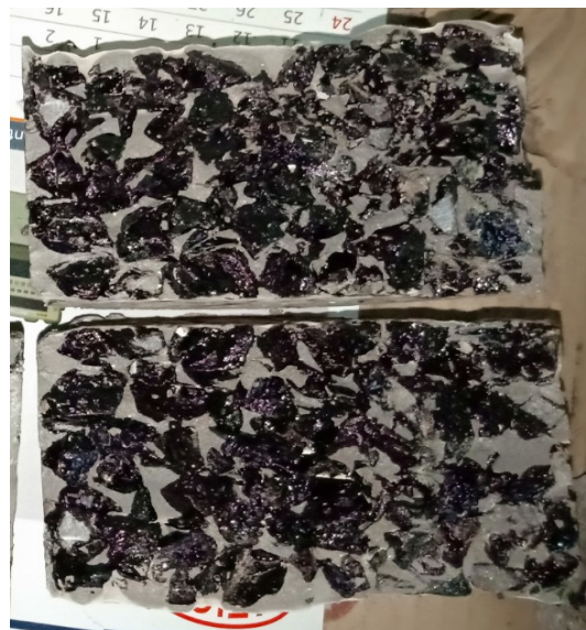
Photo 4.16. Extent of Grout Penetration in PMB 40 mix grouted specimens.
