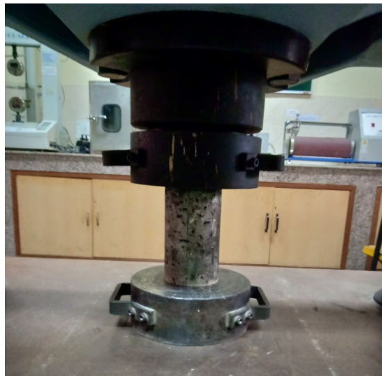
Photo 5.8. Compressive strength test
