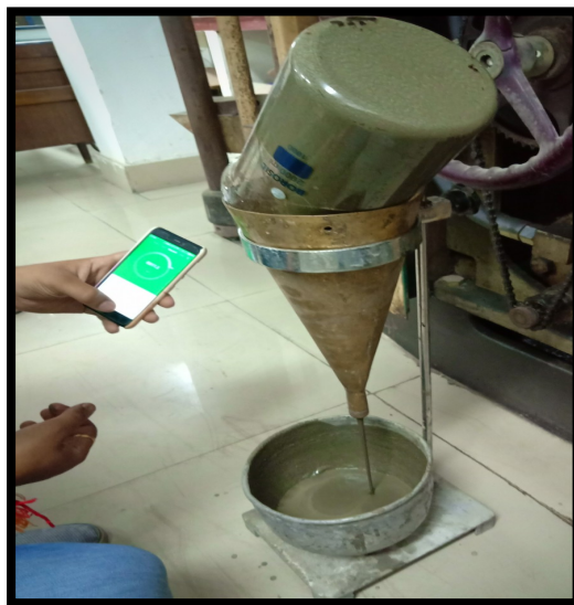
Photo 3.11 Measurement of marsh flow time for grout slurry progress
