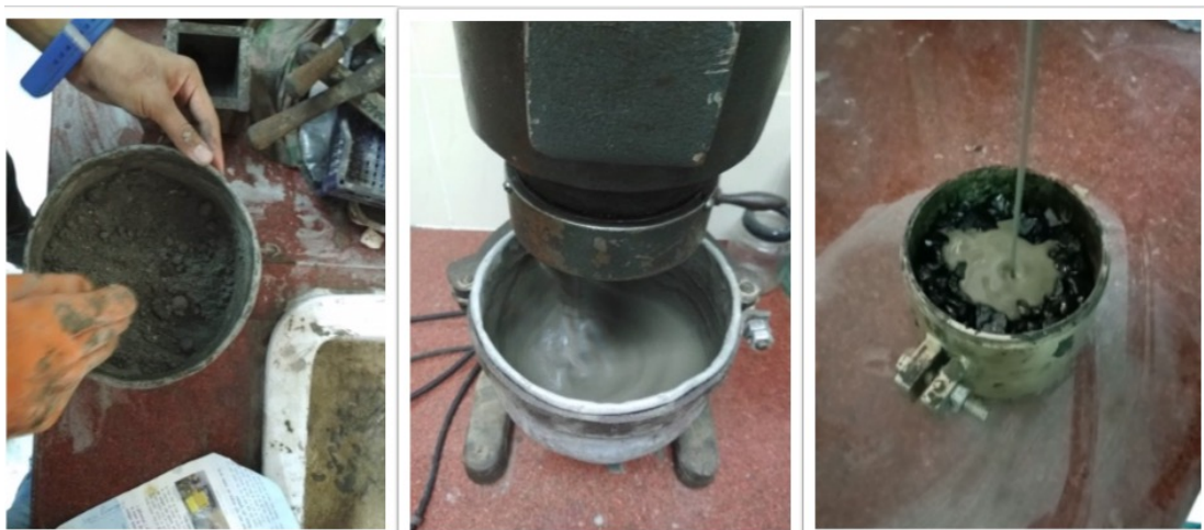
Photo. 5.1: Process of Grouting in Porous Bituminous Skeleton
