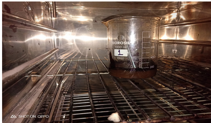
Photo 3.8: Residue test on Emulsion
