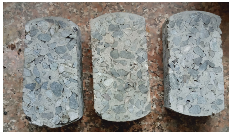
Photo 5.10. Overlay Test Specimens
