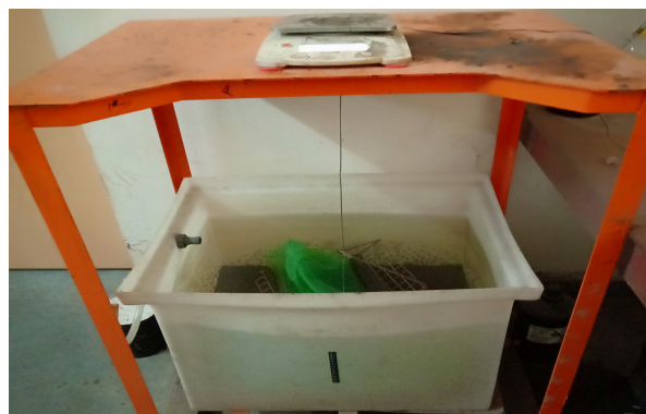
c) Weight of the Loose mix in water.
