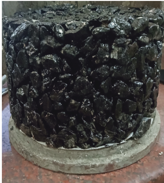
Photo 4-7. Modified High Void Bituminous mix Skelton of CGBM GR-I gradation
