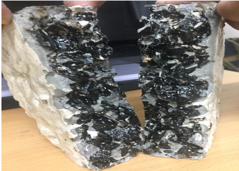
Photo 4.15. Extent of grout penetration in Emulsion mix grouted specimens
