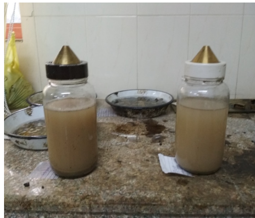
Photo 3.5: Specific gravity and W/A measurement for Fine Aggregates
