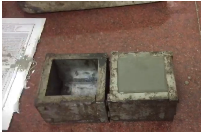
Photo 3.14. Casting of Cubes for Strength test
