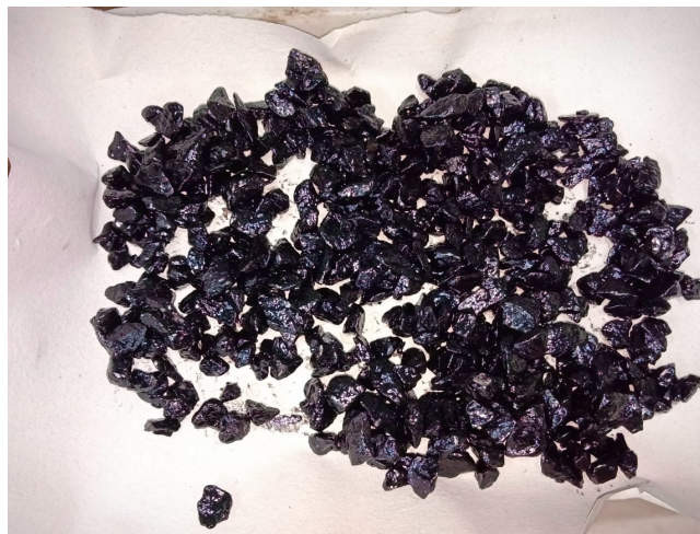
Photo 4.3. Level of coating of aggregates at Optimum Emulsion Content
