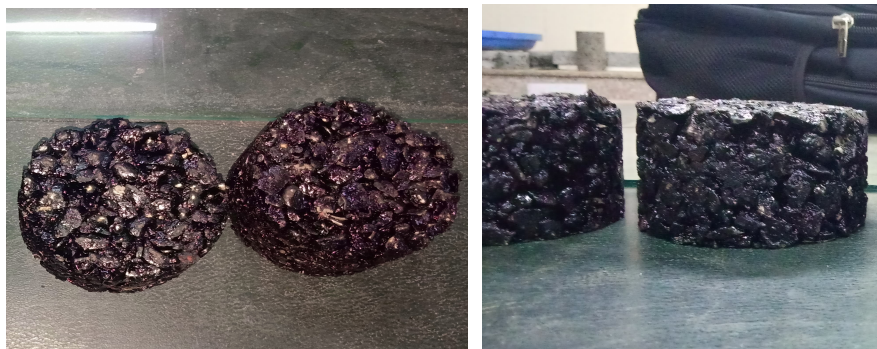
Photo 4.5. Compacted Mix of OGFC Gradation
