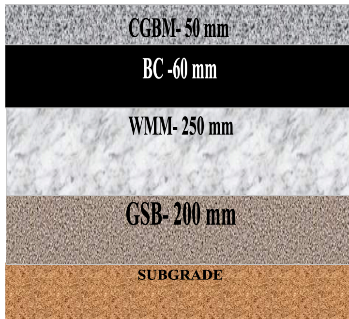
Figure 7.3. Pavement Crust Composition for CGBM
