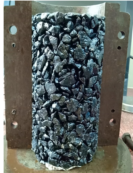
Photo 4.9. High Void Bituminous Skeleton for compression test compacted using Gyratory Compactor
