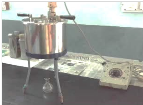
Photo 3.9: Saybolt Furol Viscosity test
