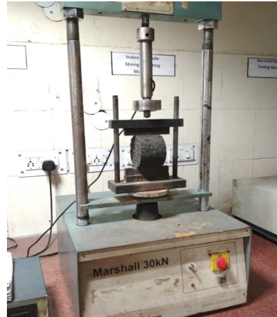
Photo 5.4. Test Setup of ITS
