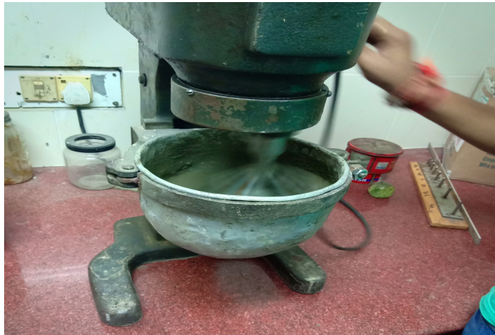
Photo 3.13. Mechanical mixing of Grout slurry
