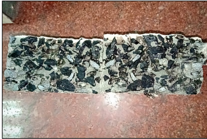
Photo 4.13. Full depth grouting at 20% W/c for CGBM GR-I.
