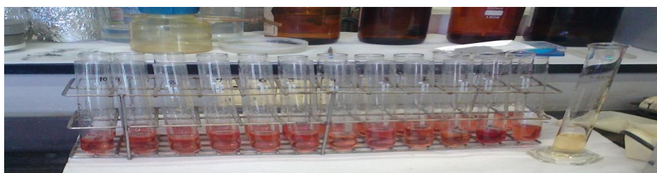
Fig. 9: Spectrophotometric method for detection of phenol
