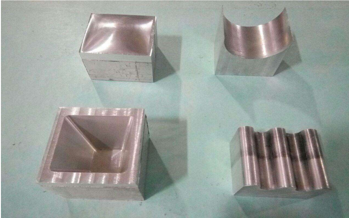
Figure 3.10: Parts Fabricated by VMC
