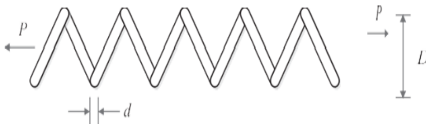
Fig. 4.7. Tension/compression spring problem schematic view
