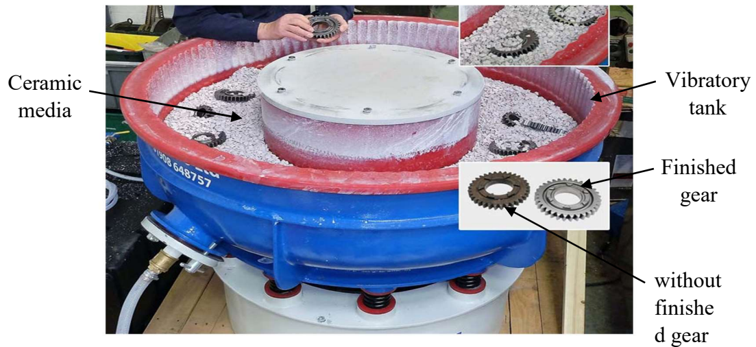
Figure 1.9 Chemical accelerated vibratory gear finish machine [17]
