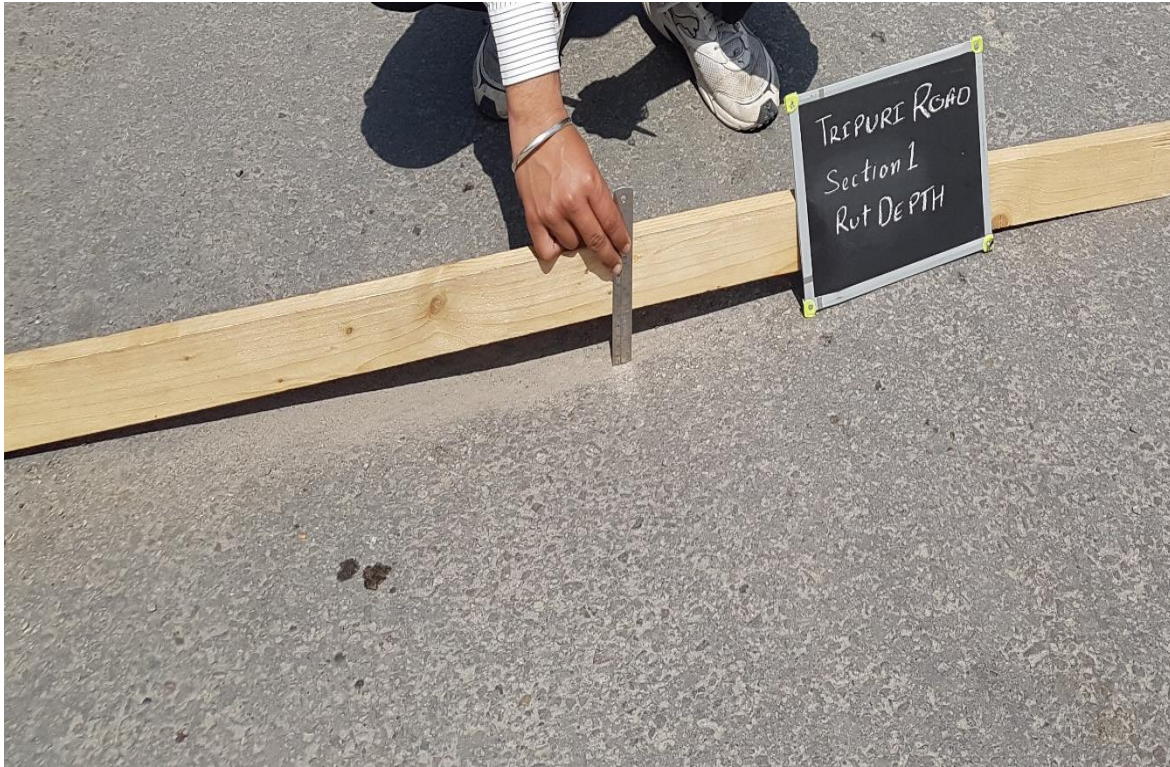
Figure 4.14: Rut Depth Measurement at Section TR
