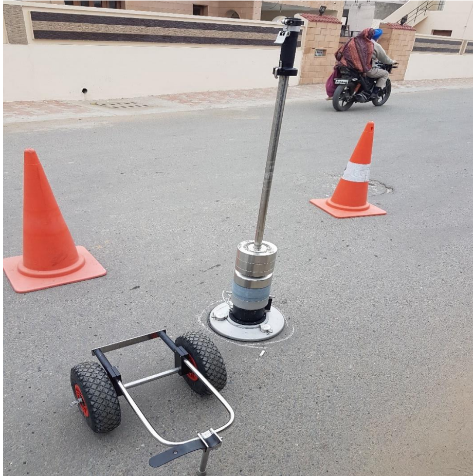
Figure 4.1: LWD Apparatus with Wheel Assembly
