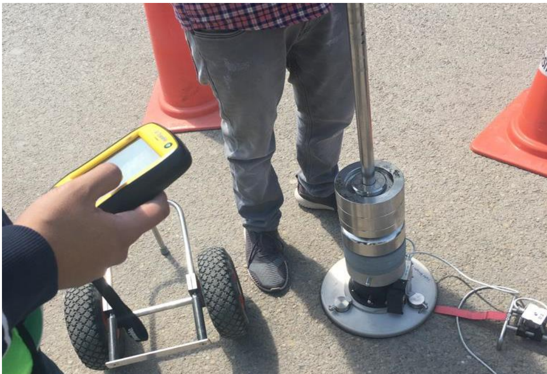
Figure 4.2: LWD with Geophone Sensor
