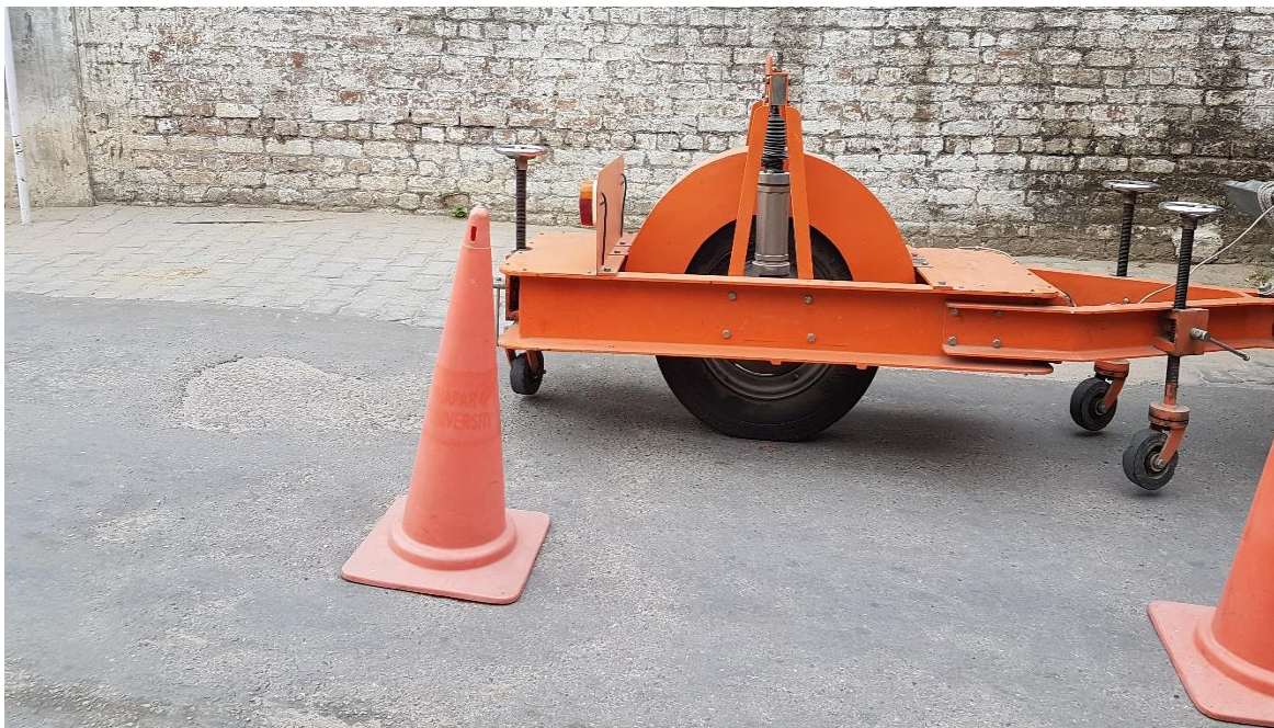
Figure 4.15: Adjusting Bump Integrator on Section LB
