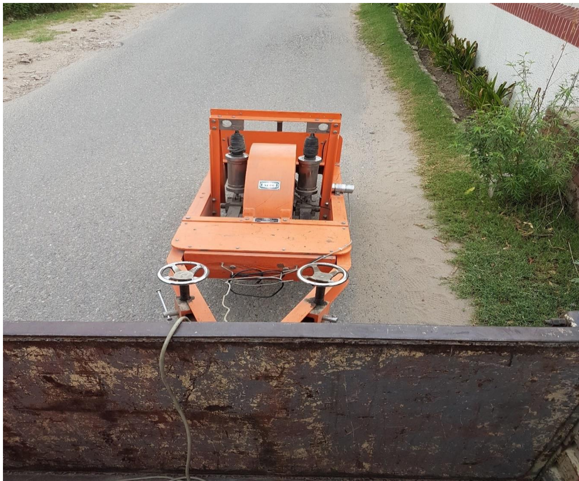
Figure 4.17: Bump Integrator Running on Section MN
