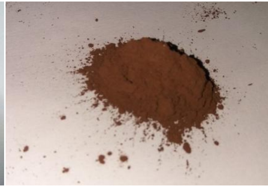
Figure 3.2 Cu-TiC powder mixtures
