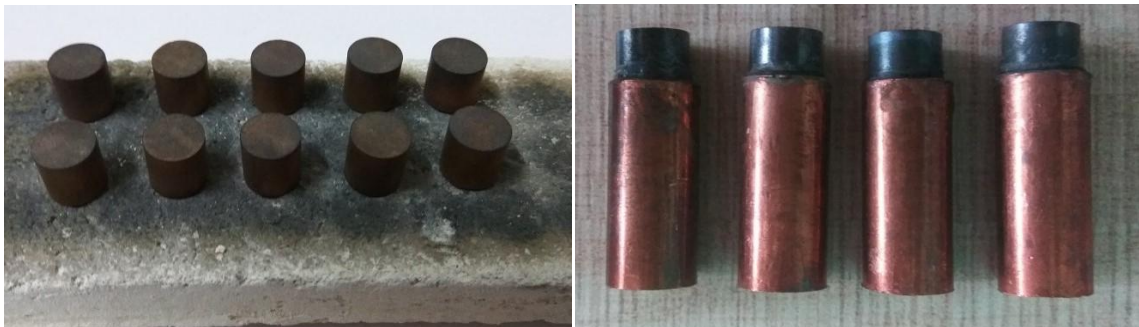
Figure 3.7 (a) Sintered Cu-TiC pallets (b) Final Cu-TiC tools
