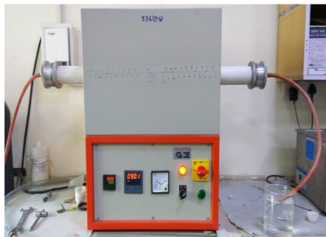
Figure 3.6 (a) Hot tabular furnace (b) Sintering cycle used in this study
