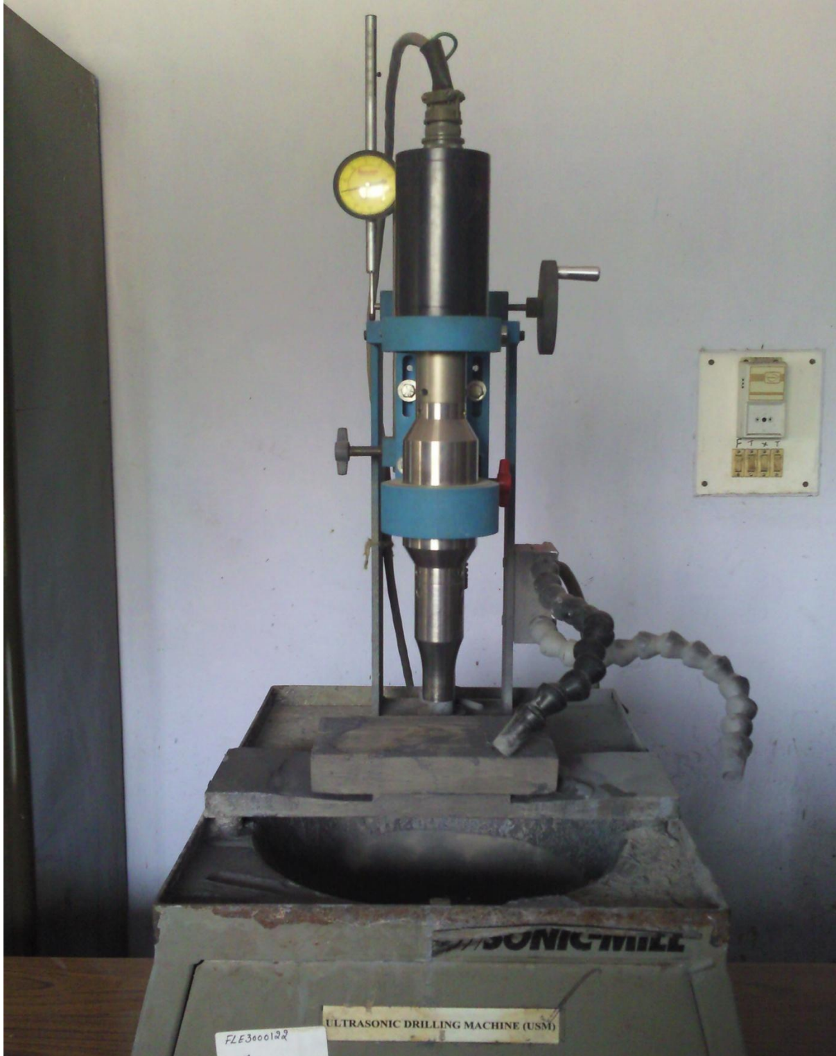
Figure 1.1 Ultrasonic Machine [N.T.M Lab, T.U, Patiala]
