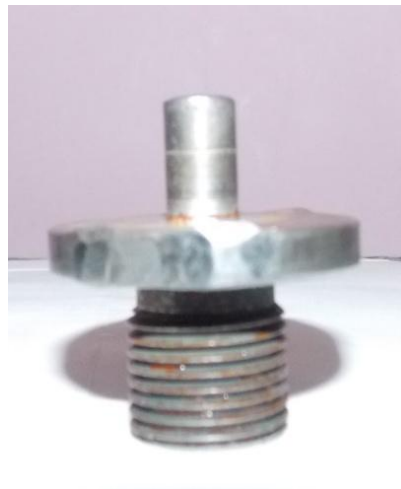
Figure 3.2 Tool Used for Ultrasonic Machining
