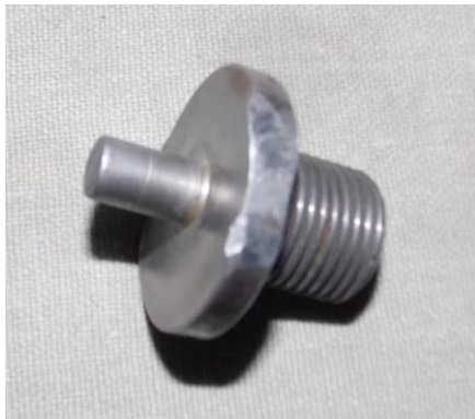
Figure 3.2 Tool Used for Ultrasonic Machining
