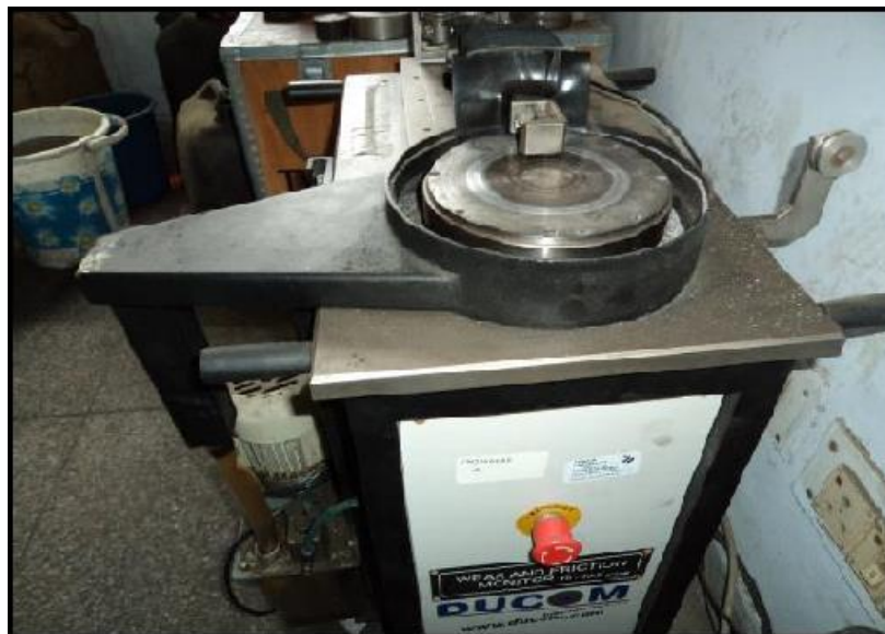
Figure 4.7: Experimental setup of wear and friction monitor (Courtesy: Machine tool Lab, TU)
