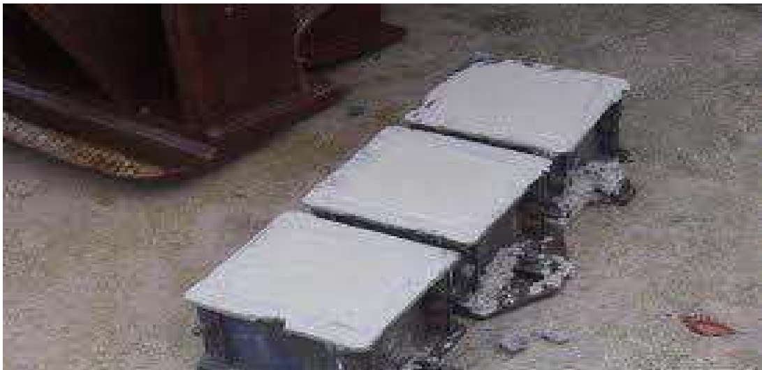
Plate 3.2: Casting of cubes
