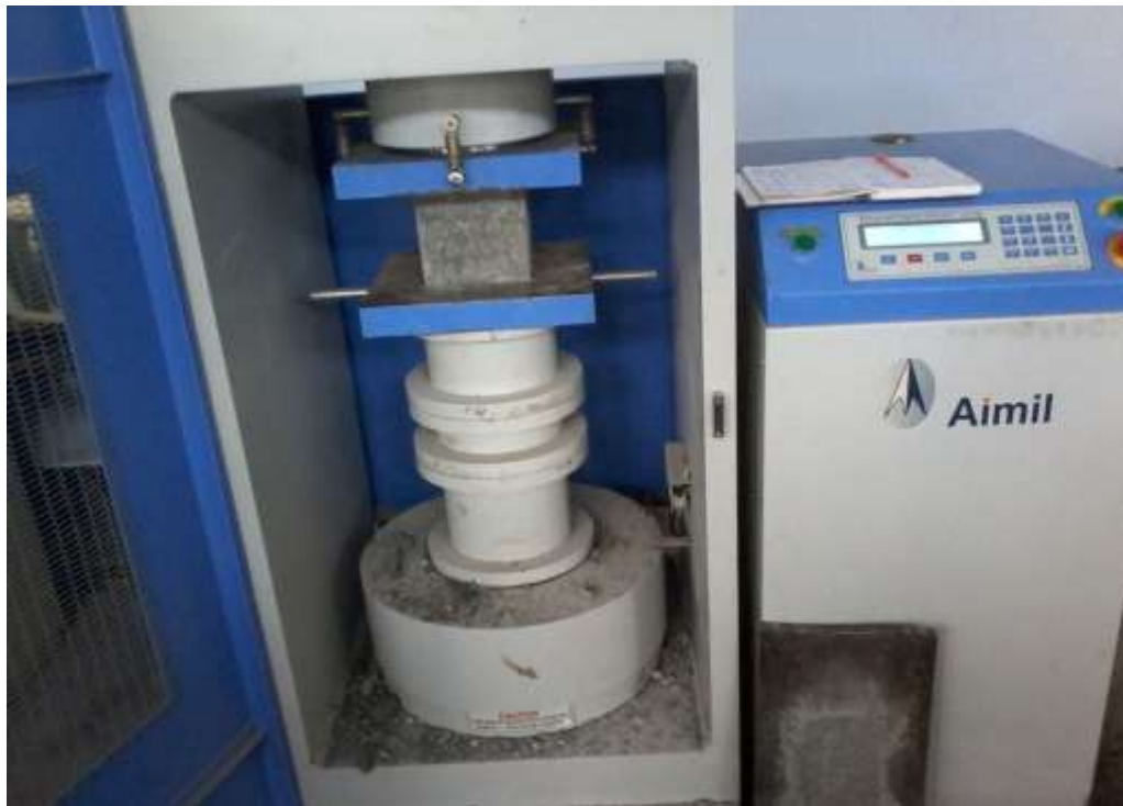
Plate 3.3: Testing for compressive strength
