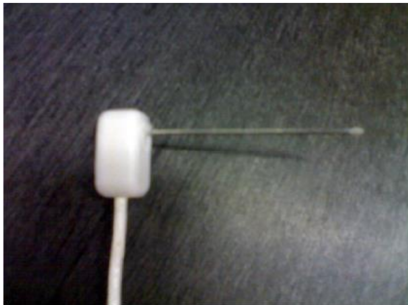
Figure 4.3: KS-1 sensor needle
