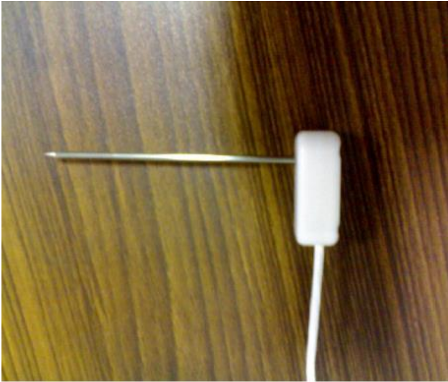
Figure 4.4: TR-1 sensor needle
