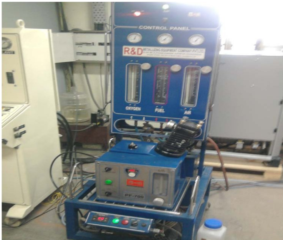
Figure 4.5 High Velocity Oxy-Fuel (HVOF) Coating Machine.
