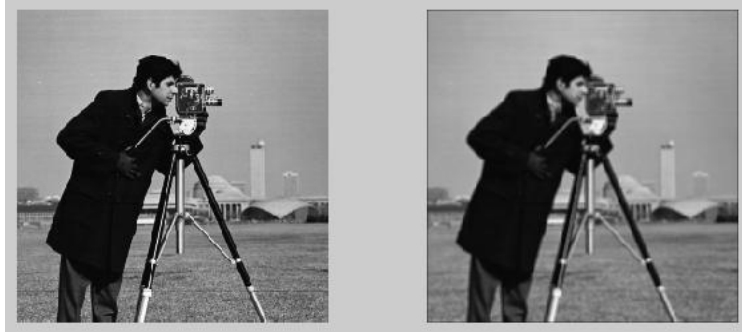
Fig 6.3: Effect of smoothing filter on image
