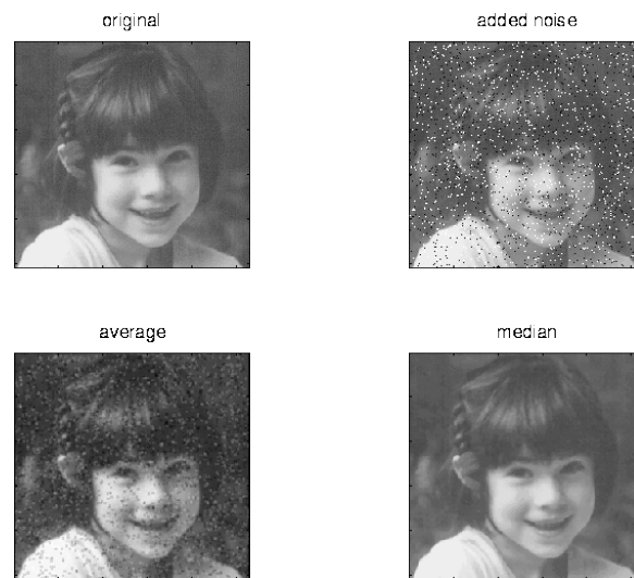
Fig 6.8 Effect of Median filtering on noisy image
