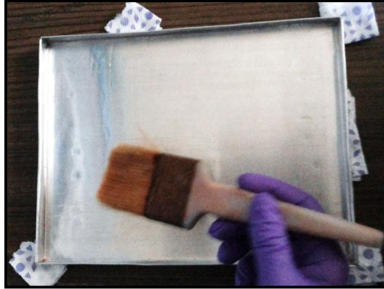
Figure 3.9: Mould Coating with Releasing Agent
