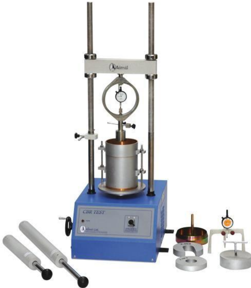
Figure 3.1: California Bearing Ratio Testing machine & equipments
