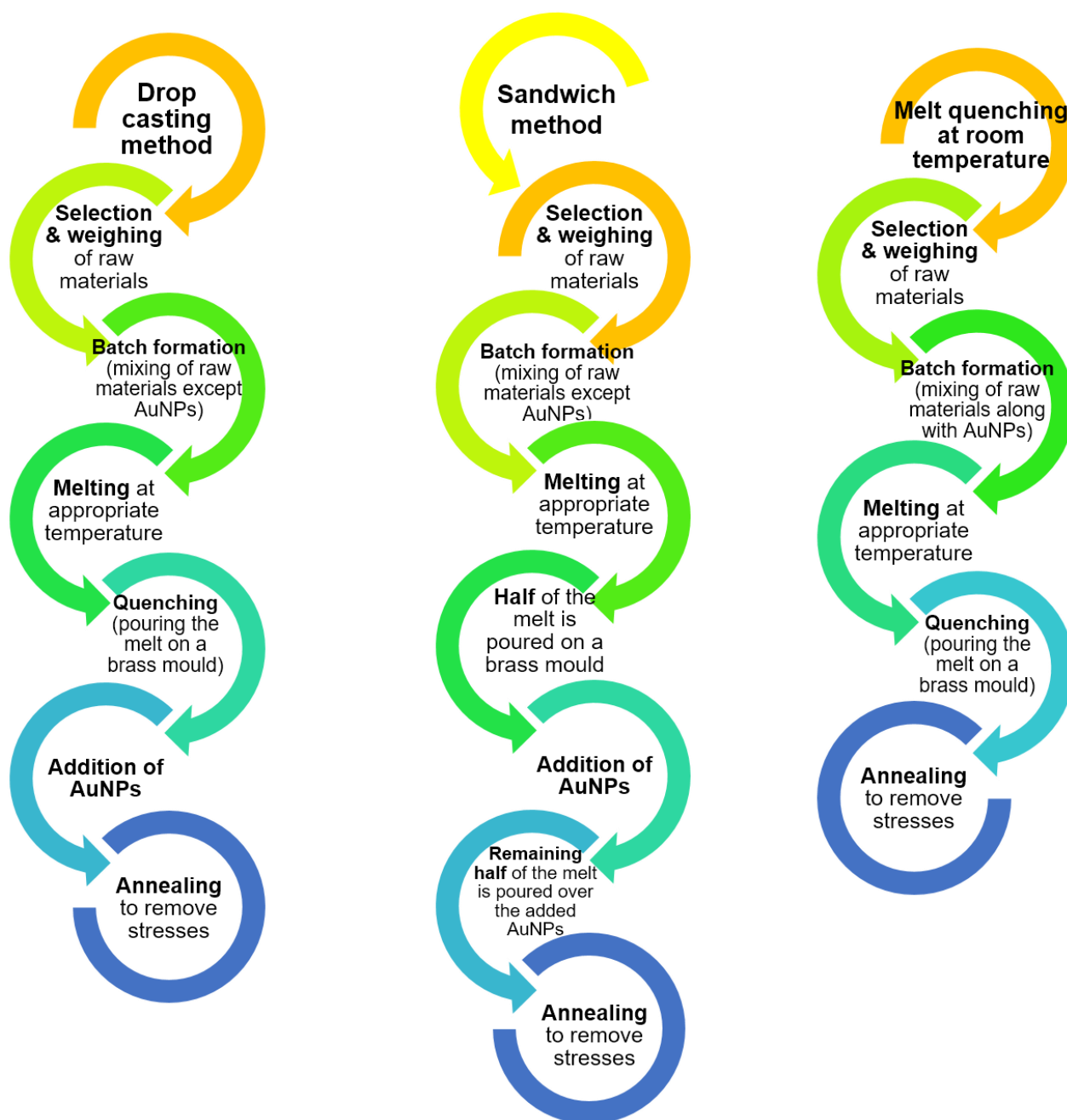
Figure 3.1: Schematic representation of all the three methods followed for the sample preparation.
