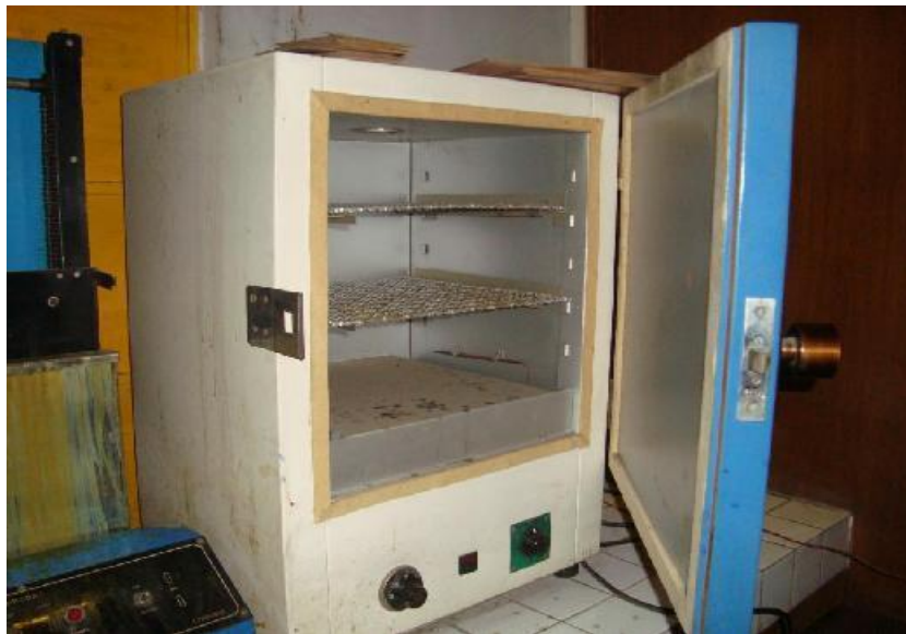
Figure 4.3 Oven unit used for drying process
