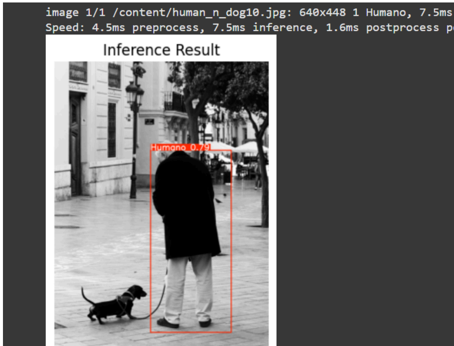
Figure 15: Human detection by the PDSC-YOLOv8n model, accurately identifying one individual with a confidence score of 0.79 in a grayscale urban scene.
