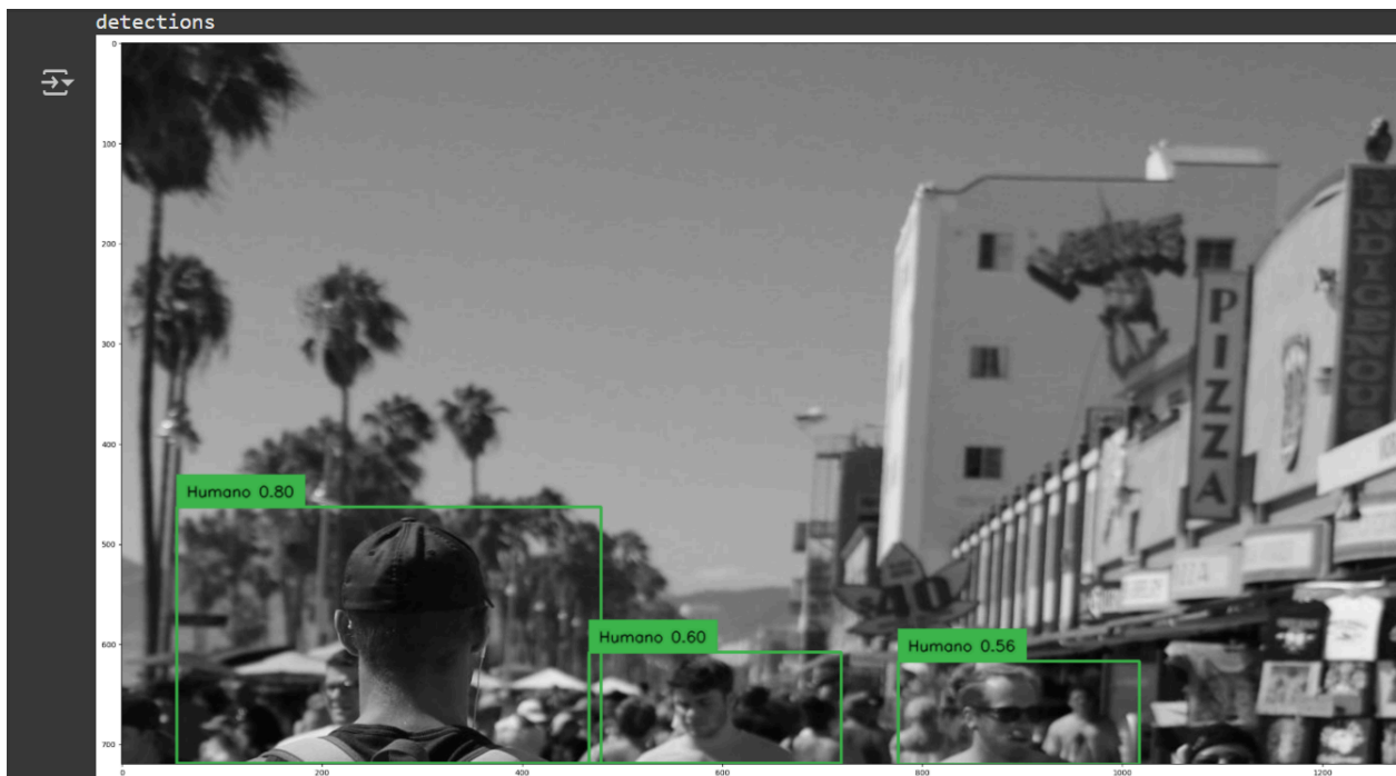
Figure 9: Actual detections by DETR-R50 with each person's probability of being a human mention above their respective bounding boxes.
