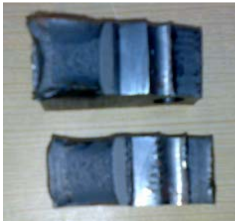
Figure 4.13 Fractured surface of broken CT specimen.
