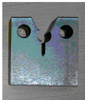
Figure 4.8 CT specimen used for testing
