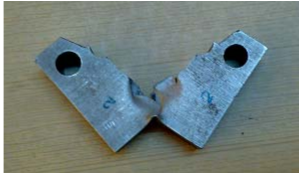
Figure 4.12 Fractured CT specimen.
