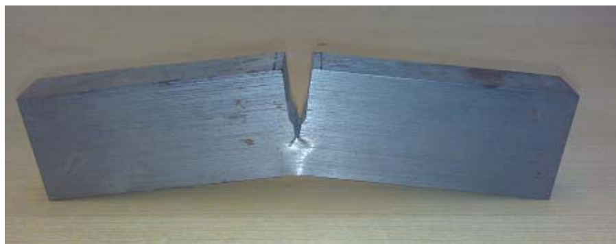
Figure 4.14 Fractured TPB specimen.
