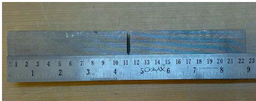
Figure 4.10 TPB specimen used for testing
