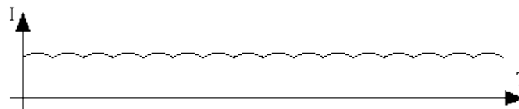
Fig. 2.16 Current output of ideal motor
