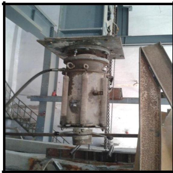
Fig 3.6 Hydraulic operated jack
