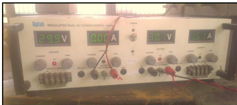
Fig 3.4 DC Regulated Dual Power Supply Source(constant voltage)
