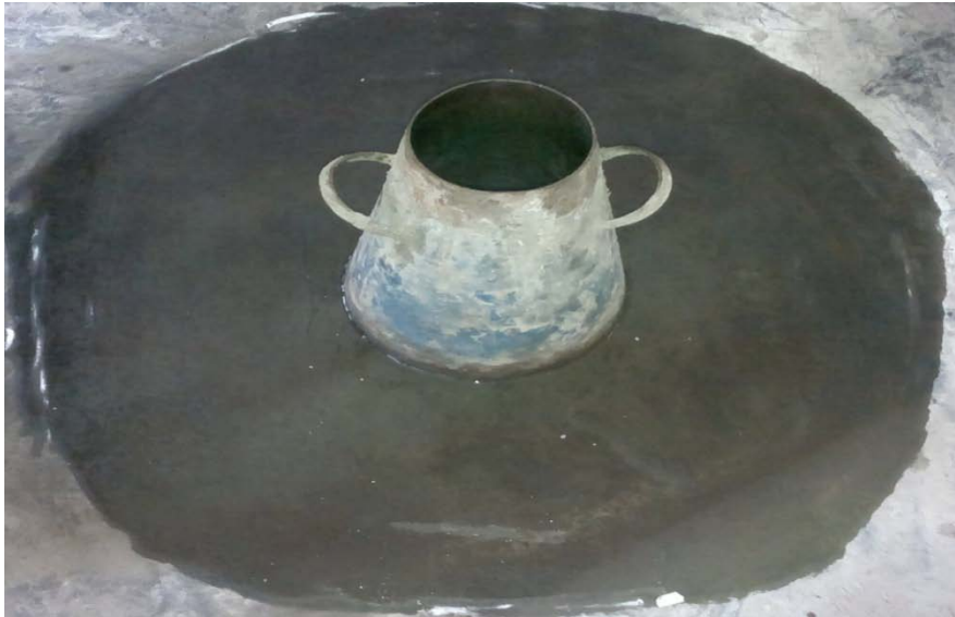
Fig. 4.1 Slump flow test conducted for self-compacting concrete
