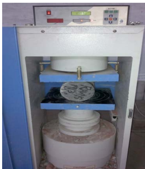
Fig. 3.8 Splitting Tensile Strength
