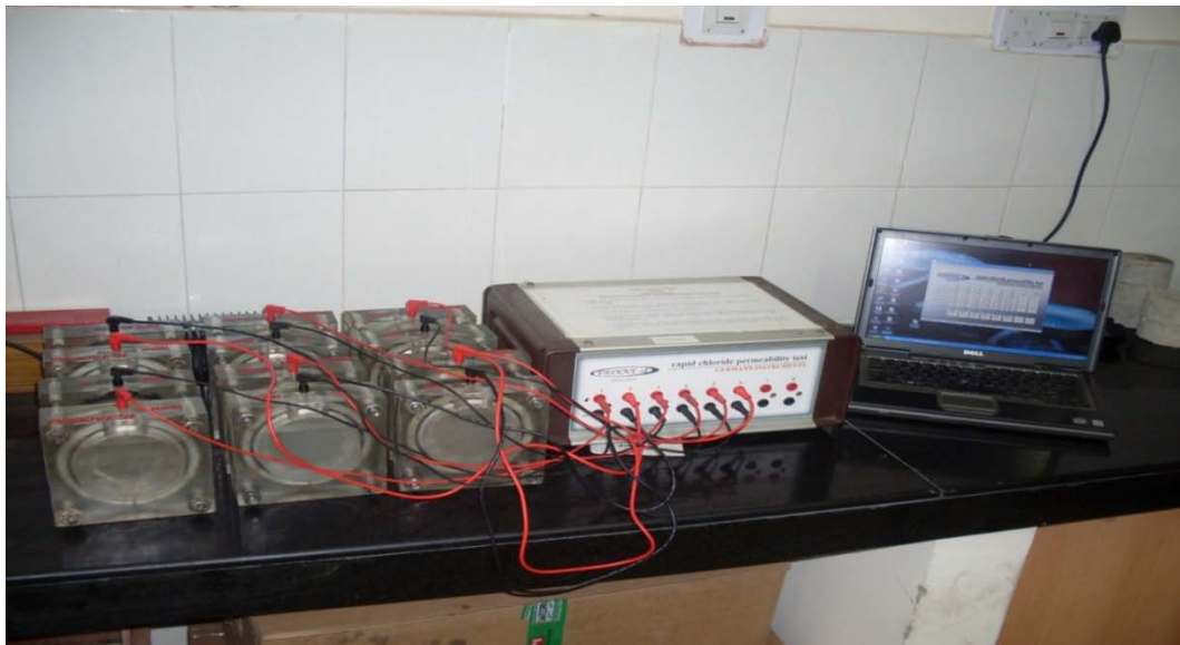
Fig.3.9: Rapid chloride permeability test set up (ASTM C 1202).
