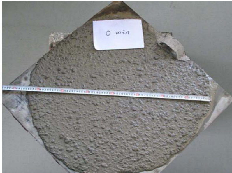
Fig. 1.7: Slump flow test (Zhimin et al. , 2008)
