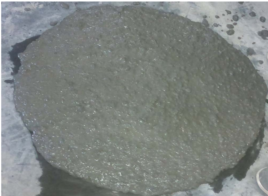
Fig.4.2 Slump flow test
