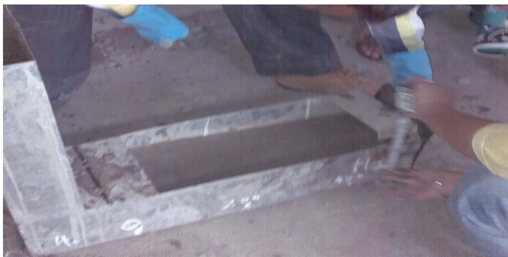
Fig.4.5: L-Box test in progress
