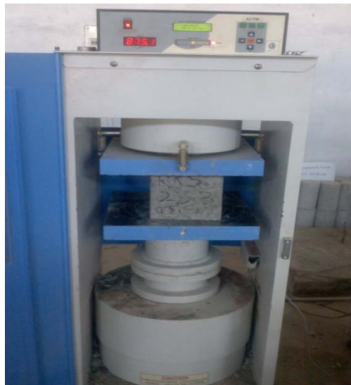
Fig. 3.7 Compressive Strength Test
