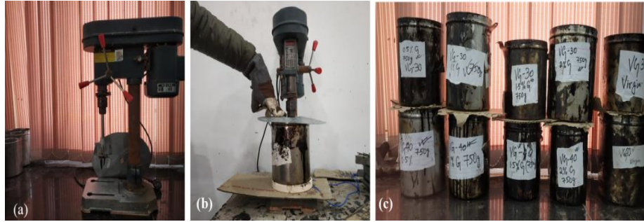
Figure 11 (a) Make Shift Mixer (b) Mixing with a Metallic Lid (c) Ten Samples of 750 g each Produced
