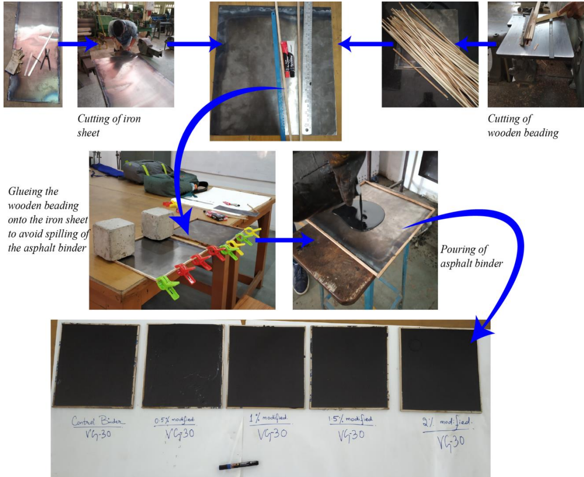
Figure 24 Sample Preparation For Thermal Conductivity Test
