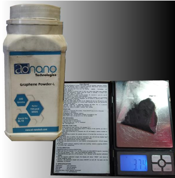
Figure 26 Graphene Container and Weighing Scale with 0.5% Graphene by Weight of 750 g Asphalt
