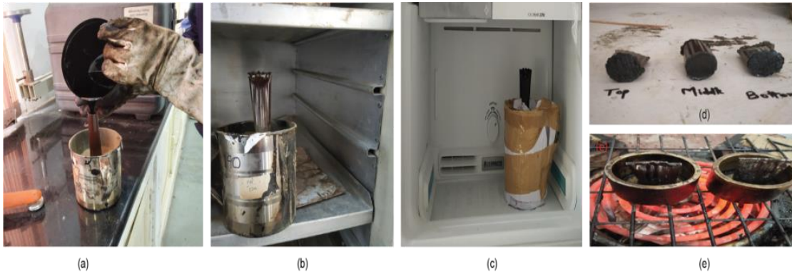
Figure 13 (a) Pouring of Asphalt Binder into the Tube (b) Shifting the Sample in the Oven for 24 Hours (c) Freezing the Sample in the Freezer to Stabilize the Constituents (d) Cutting the Sample into Three Equal Pieces (e) Heating the Top and the Bottom Half to Perform Ring and Ball Test
