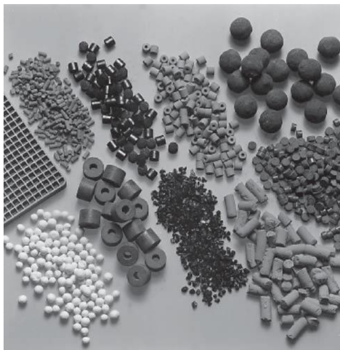
Figure 6 Shapes of catalysts (BASF, Ludwigshafen, Germany).
