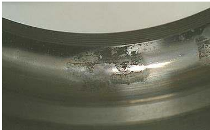
Figure 1.5 Deep seated rust in outer ring of a deep groove ball bearing [4]
