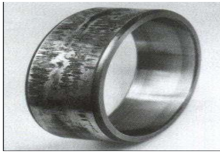
Figure 1.6 Smeared outer race of spherical roller bearing [5]
