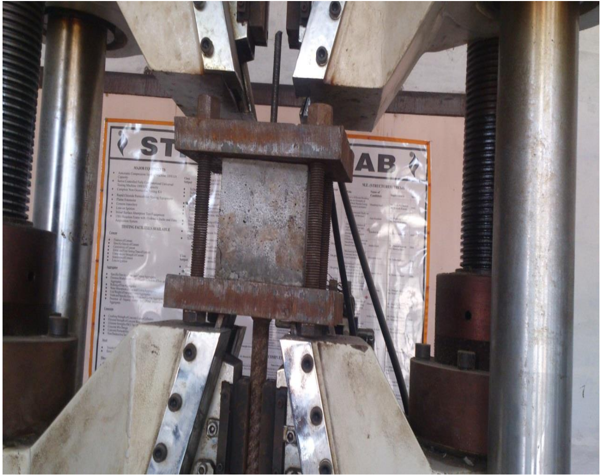
Figure 3.9: Test Setup for Pull Out Strength Test
