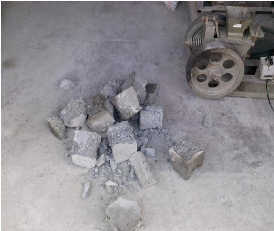
Figure 3.1: Waste Concrete Rubble for obtaining RCA
