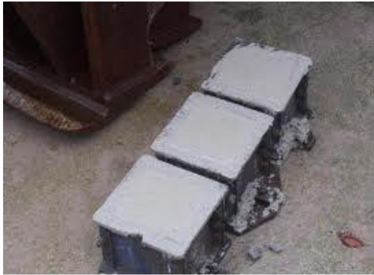
Figure 3.3: Casting of cubes
