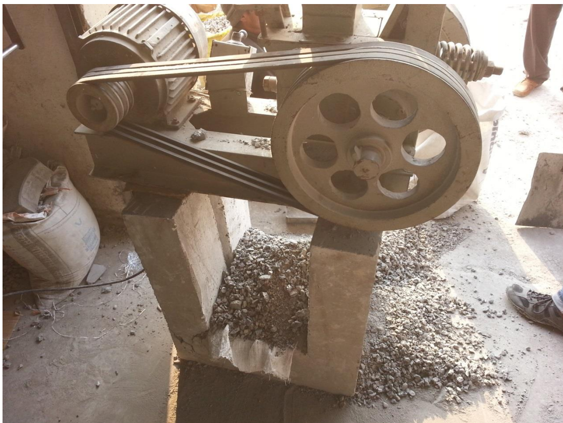
Figure 3.2: Jaw Crusher to obtain RCA
