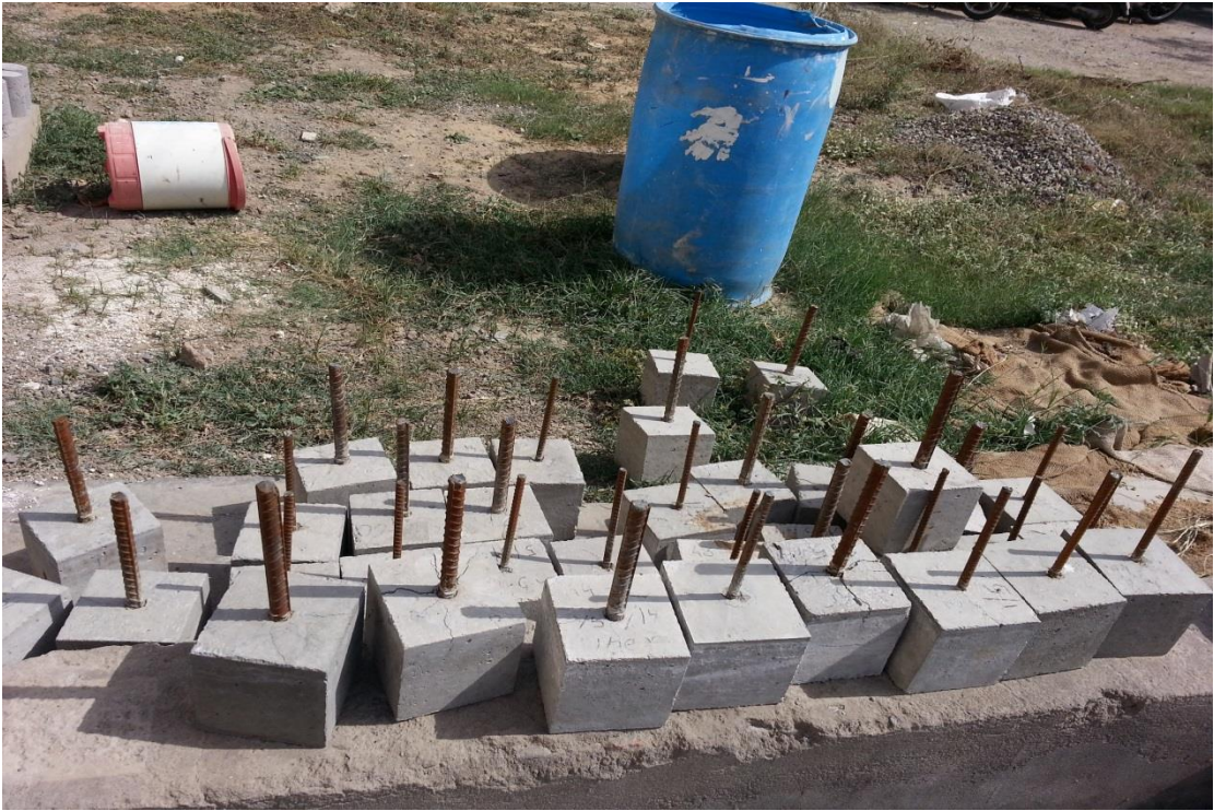
Figure 3.4: Pull out Test Specimens
