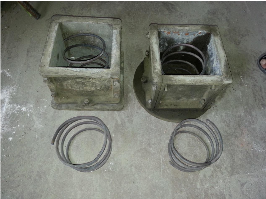
Figure 3.5: Helical Reinforcement as per IS: 2770 (Part 1)
