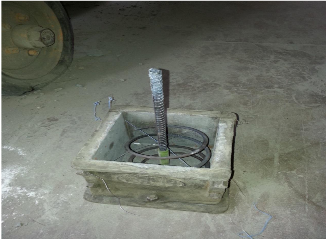
Figure 3.6 Arrangement of the Mould Before Casting
