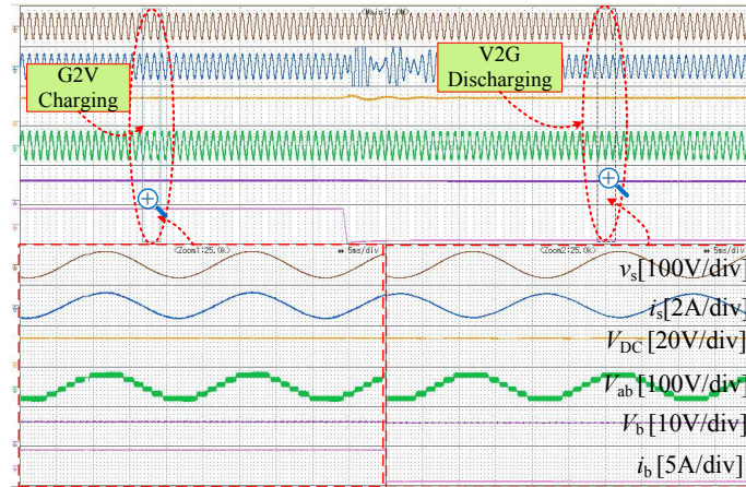
Fig. 5.9: Sudden change in G2V charging to V2G discharging mode
