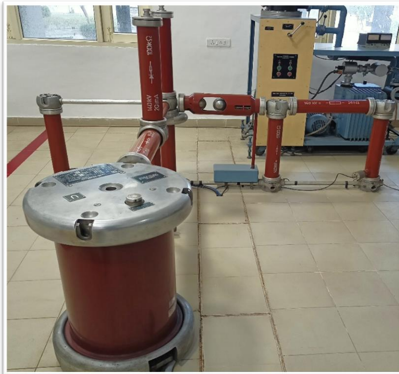
Figure 4.2 Impulse generator kit used to measure impulse voltages.
