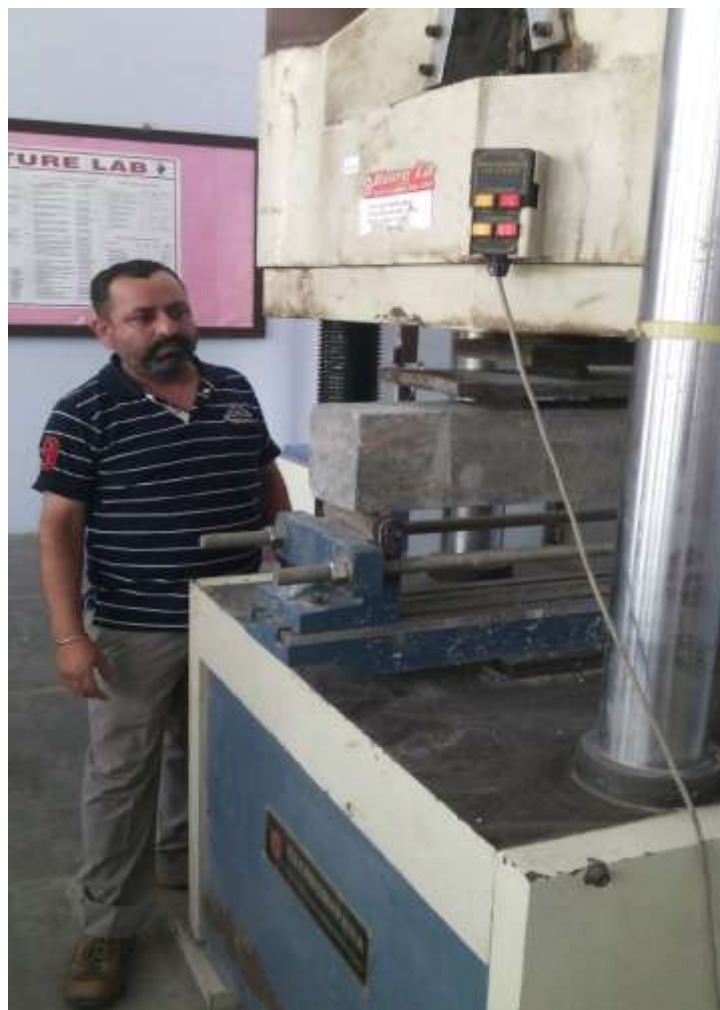
Fig. 4.8 Test for Flexural Strength of Concrete
