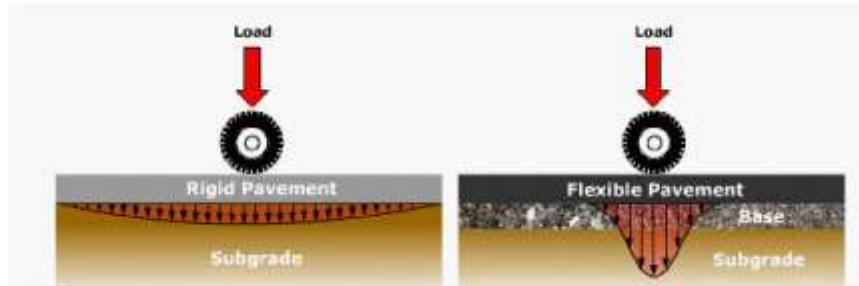
Figure 1.7. Typical stress distribution under a rigid and a flexible pavement.
