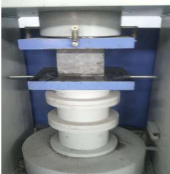
Fig. 4.1 Test for Compressive Strength of Concrete
