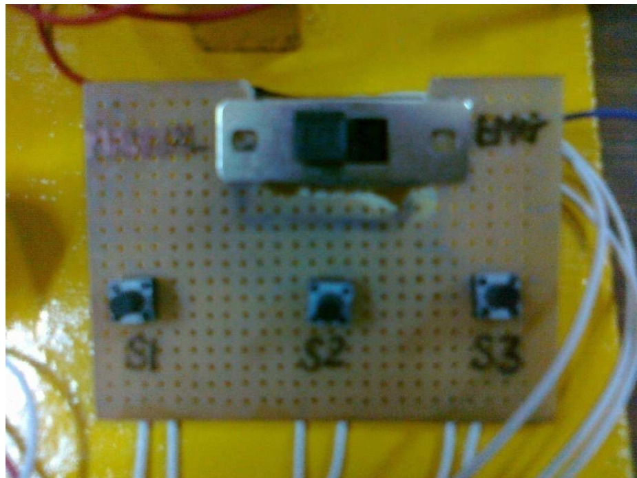
Figure 4.1: Selection switch in manual position
