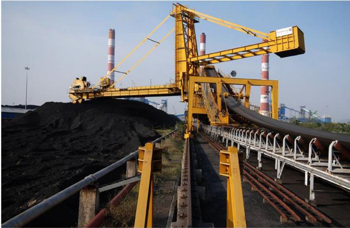
Figure 3.1 Picture of Coal handling plant of NTPC Dadri picture clicked by me at site
