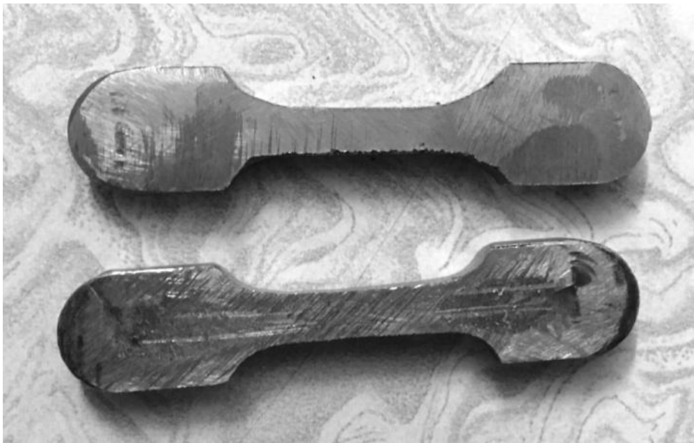
Fig. 5.8: Dog bone shape tensile test specimens as per ASTM (E8M) standards
