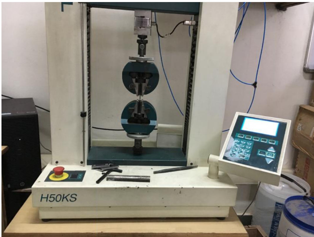
Fig. A-6: Universal tensile testing machine (Courtesy: Mechanical Engg. Dept., IIT Ropar)
