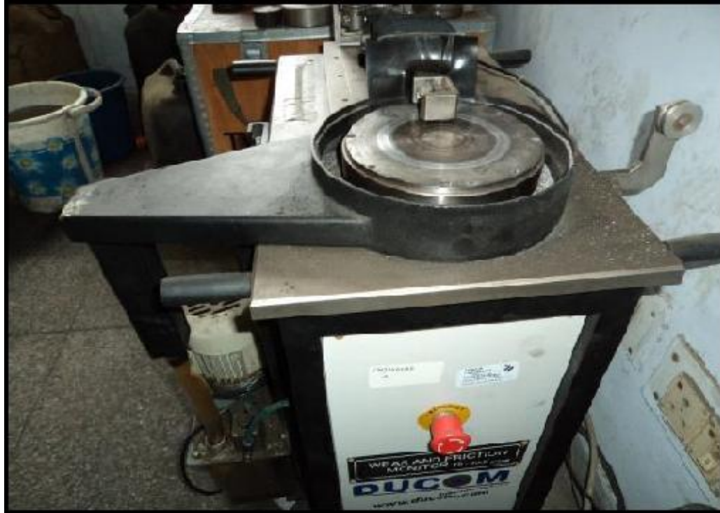
Fig. A-7: Pin on disc tribometer (wear and friction monitor) (Courtesy: Tribology Lab, Thapar Institute of Engineering & Technology)
