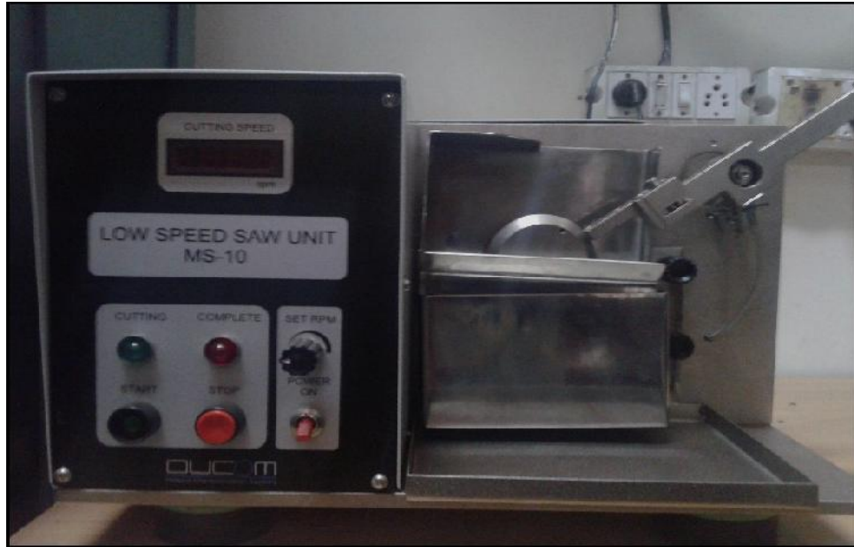
Fig. A-1: Low speed diamond cutter (Make: DUCOM, Model: MS-10, Courtesy: Microwave materials processing lab, Thapar Institute of Engineering & Technology)
