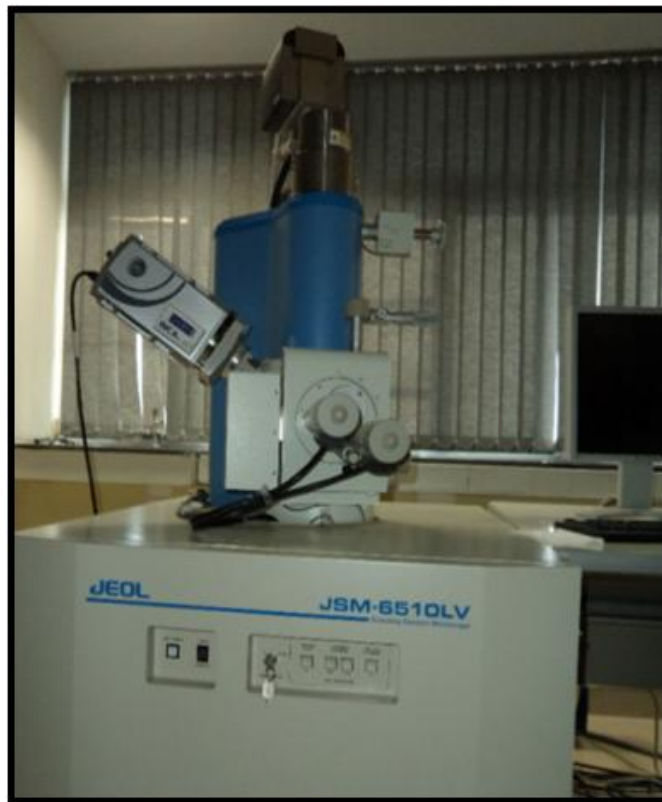
Fig. A-4: Scanning Electron Microscope (Courtesy: SAI Labs, Thapar Institute of Engineering & Technology)
