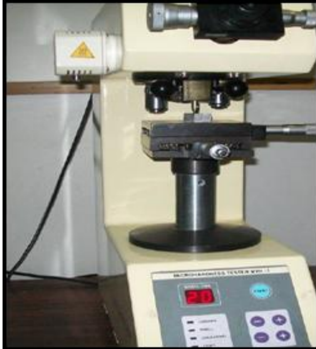
Fig. A-5: Vickers Micro-hardness Tester (Courtesy: A.M. Lab, Thapar Institute of Engineering & Technology)
