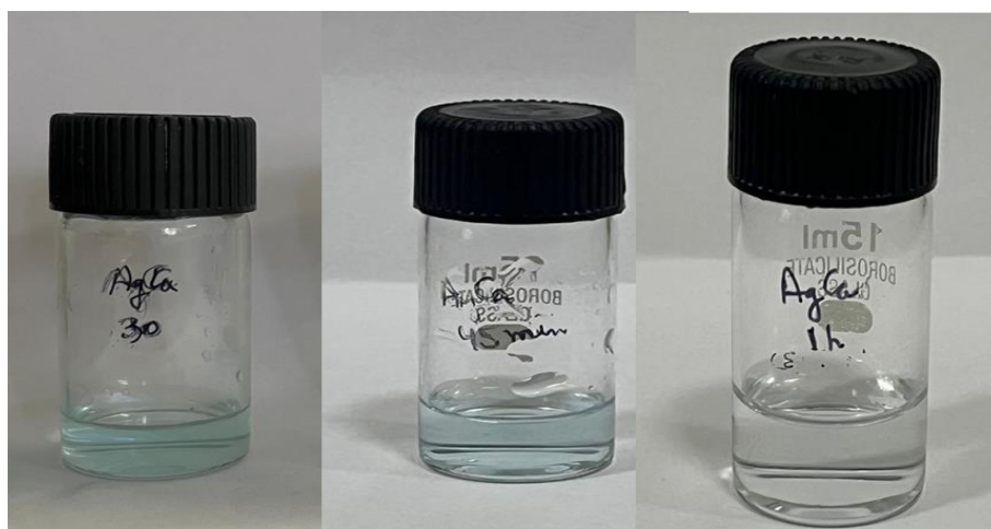
Fig.22: Degradation of MB dye by Ag-CaTiO 3 under sunlight
