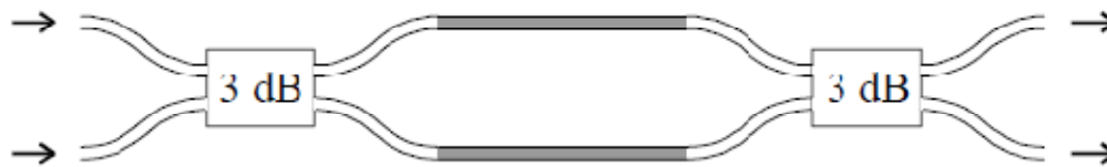
Fig 1.5 Mach-Zehnder interferometer based switch
