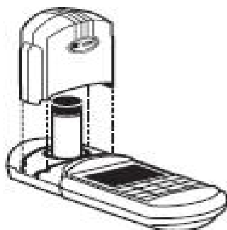
Fig 3.7: HACH DR 890 colorimeter with sample cell
