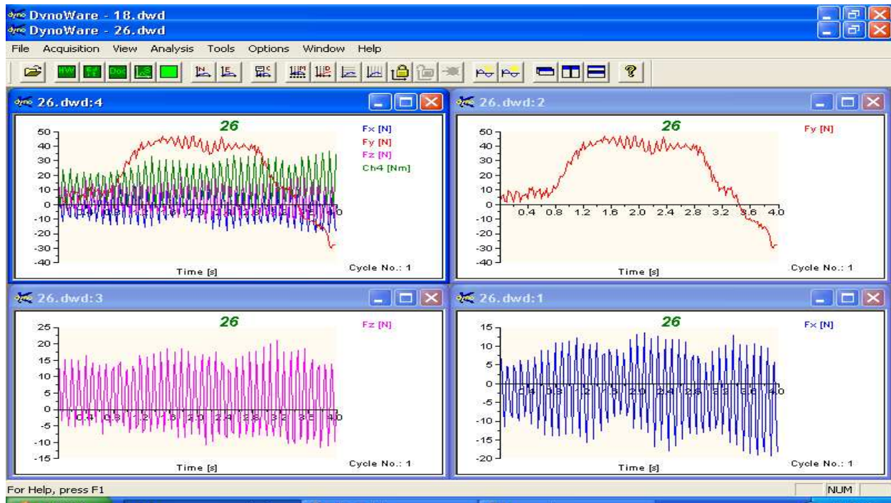
Fig. 3.36 Graphical representation for feed .2mm/rev., speed 580 rpm and point angle 118°
