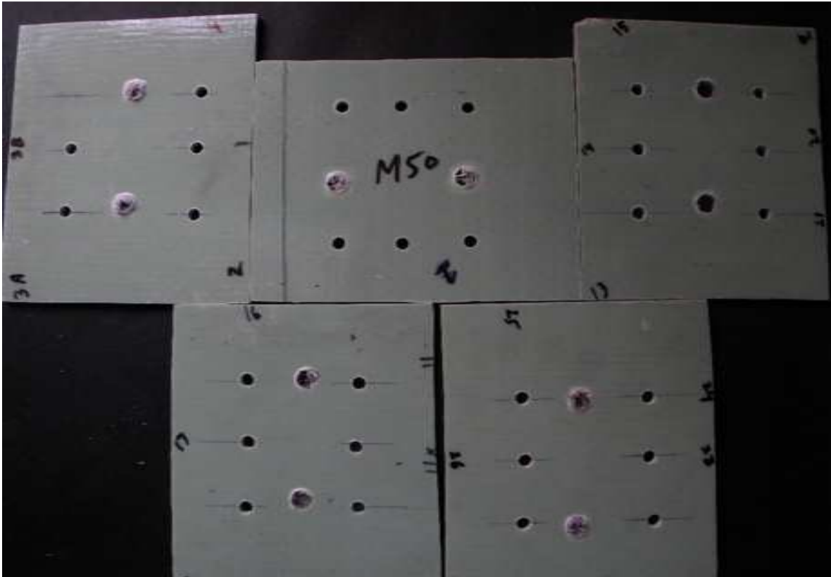
Fig.3.39 Specimens drilled with M50 twist drill
