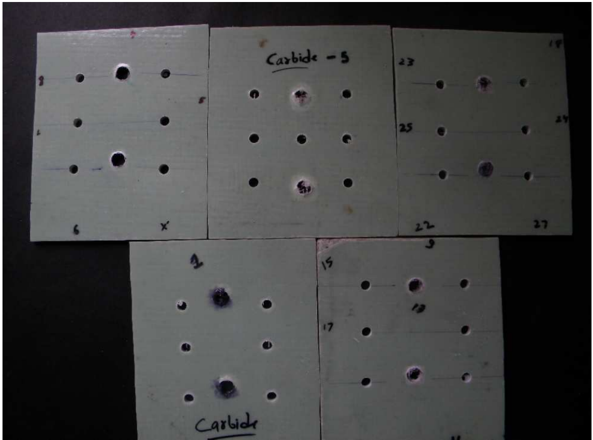
Fig.3.10 GFRP drilled by tungsten carbide drill bit
