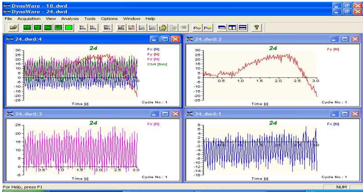
Fig. 3.34 Graphical representation for feed .1mm/rev., speed 890 rpm and point angle 118°
