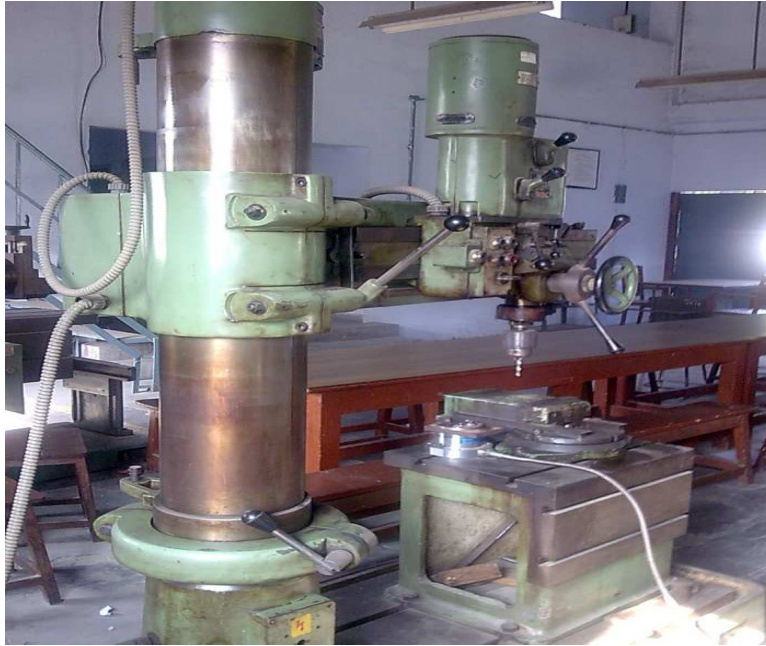
Fig. 3.6 A radial drilling machine
