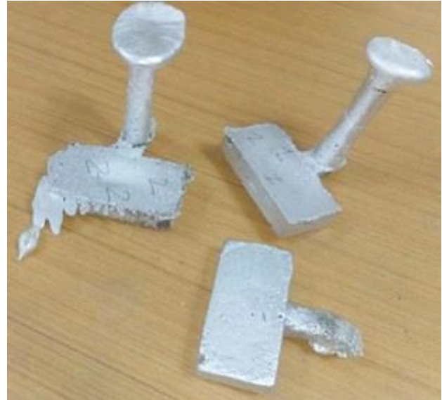
Figure 3.12: Composite casting of desired shape
