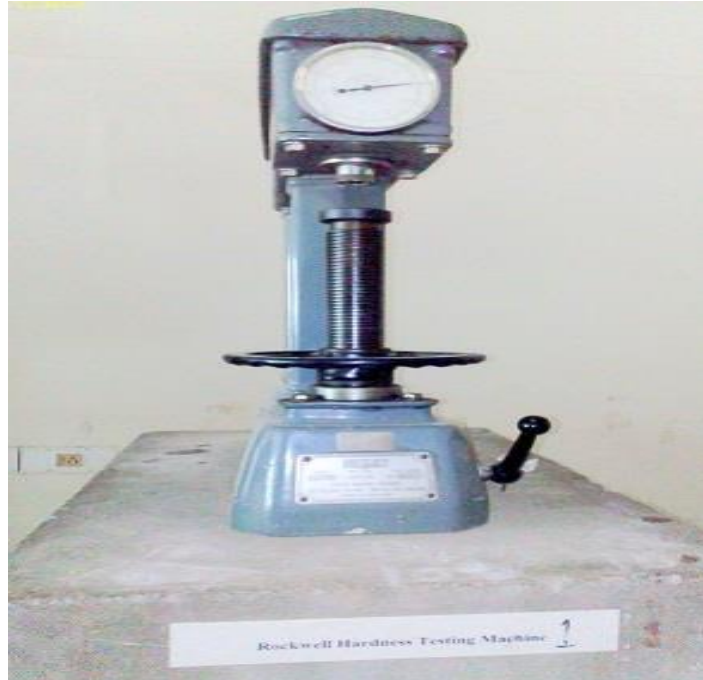
Figure 3.13: Rockwell hardness testing machine (Courtesy: Strength of Material Lab, Thapar University, Patiala)
