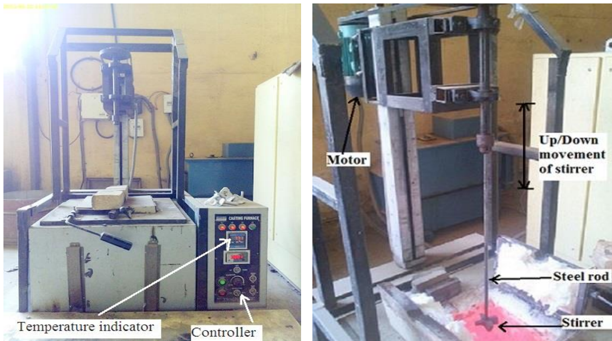
Figure 3.7: Casting furnace (Courtesy: Central Workshop, Thapar University, Patiala)
