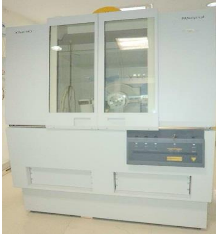
Figure 3.16: X-ray diffractometer (Photo courtesy: SAI Labs, Thapar University Campus, Patiala)
