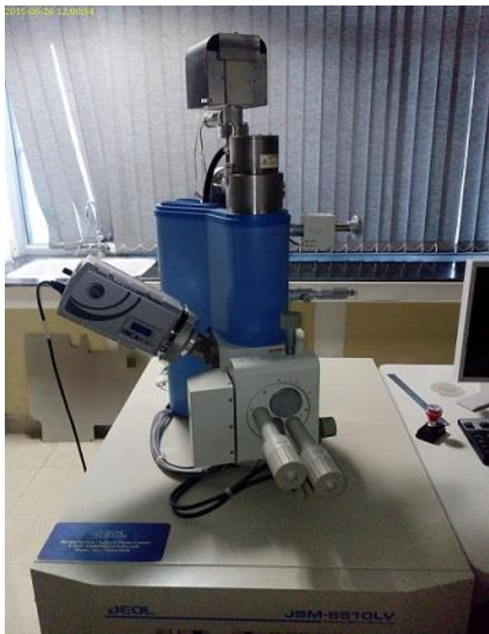
Figure 3.15: Scanning electron microscope (Photo courtesy: SAI Labs, Thapar University Campus, Patiala)
