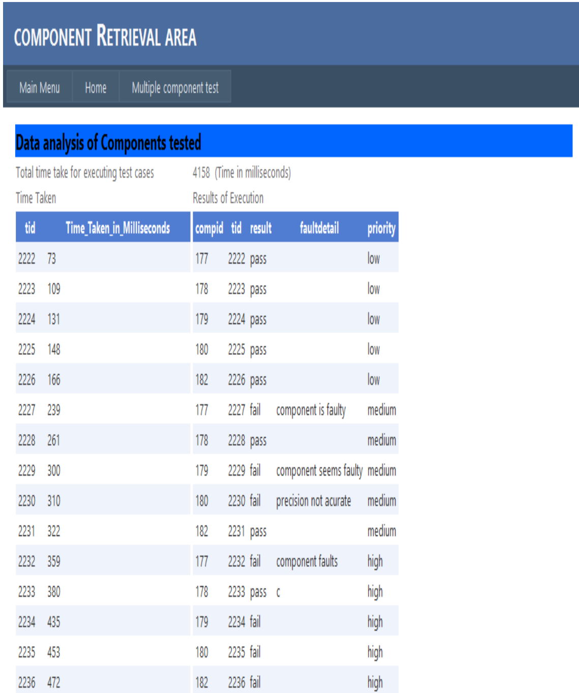
Fig. 4.12 Data analysis obtained from interface testing of COTS Components.
